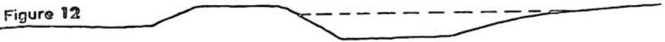
Cross section of a diversion channel in flatter country. Fall 1 in 500 to 1 in 5000.
