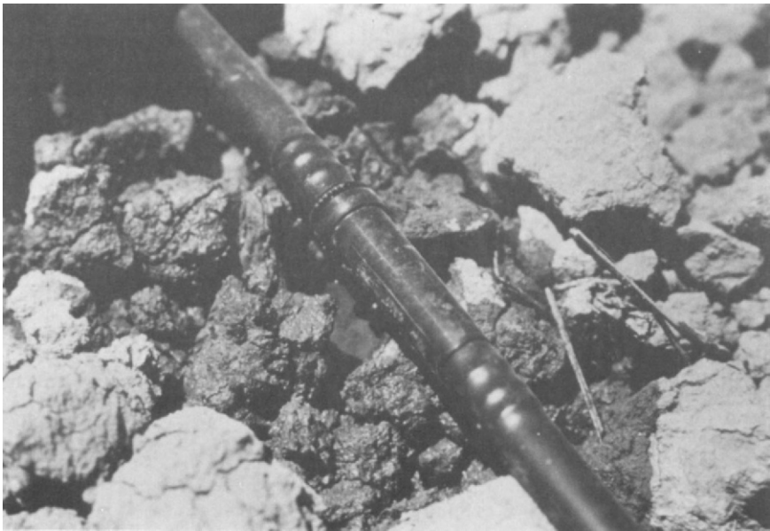
Fig. 1.1.6 Point-source emitter used for surface trickle irrigation.
