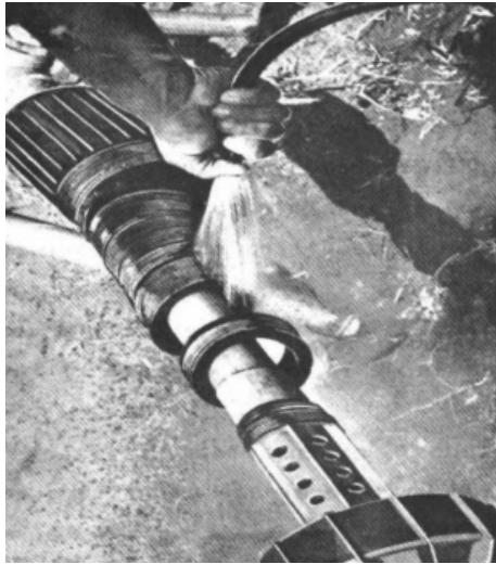
FIGURE 8 Flushing method for the disk filter.
