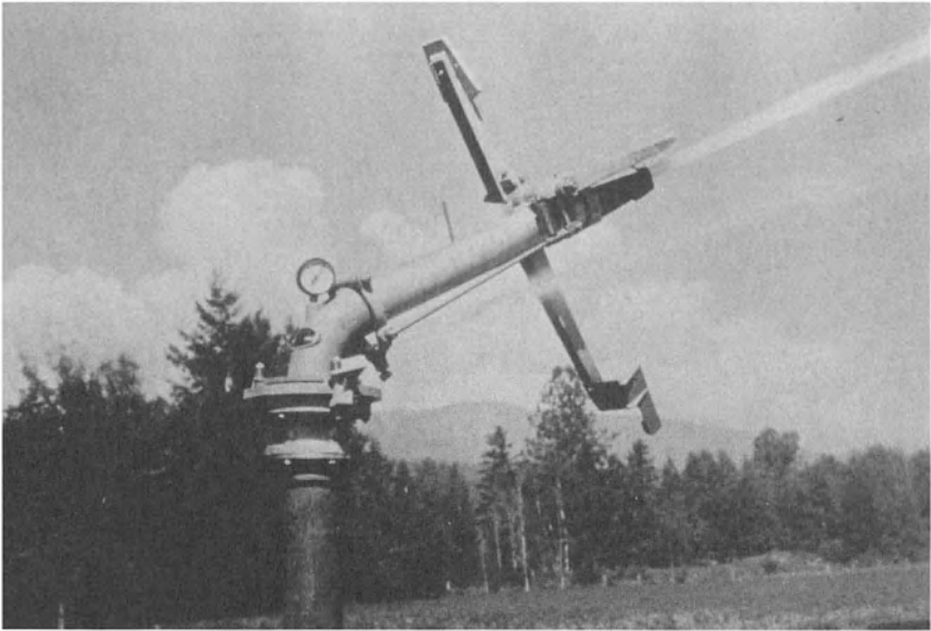
FIG. 4.4. Part-circle Gun Sprinkler with Rocker Arm Drive.
