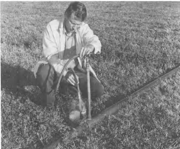
FIG. 6.3. Measuring Sprinkler Discharge Using a Hose to Direct the Water into a Container of Known Volume.
