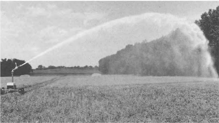
FIG. 2.3. Hose-fed Traveling-gun Sprinkler in Operation (Source: Nelson Irrigation Corp.).
