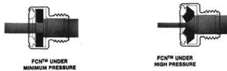
A. Nozzle Operation (Source: Nelson Irrigation Corp.).
