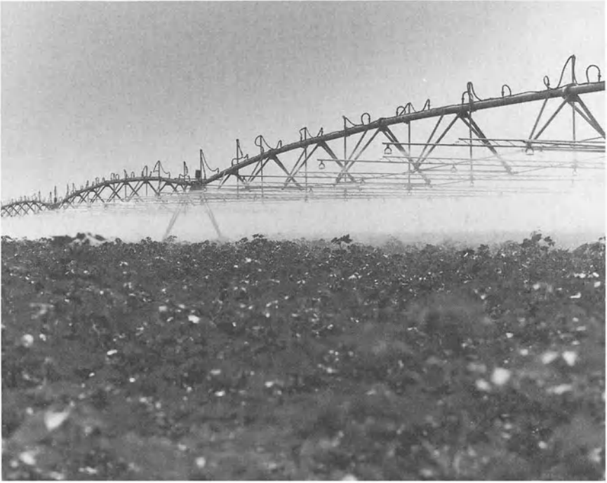
FIG. 14.5. Center-pivot Lateral With Low-pressure, Fixed-spray Sprinklers on Short Booms (Source: Nelson Irrigation Corp.).
