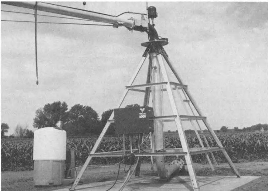
FIG. 4.10. Outer (Top) and Pivot (Bottom) Ends of Center-pivot Lateral (Source: Valmont Industries, Inc.).
