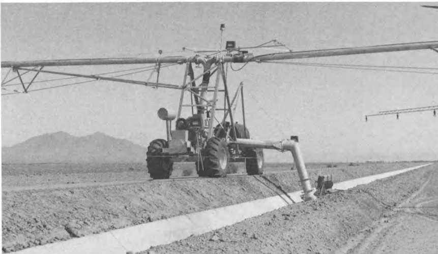
FIG. 4.12. Linear-moving System with Open Channel Water Supply (Source: Valmont Industries, Inc.).
