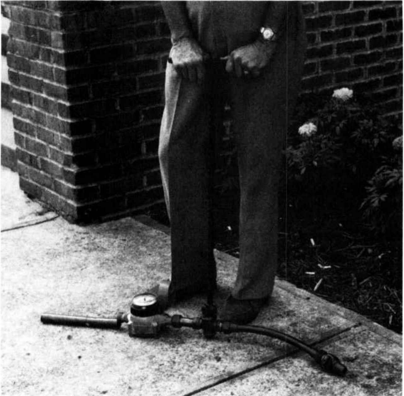
FIGURE 10.2 Water meter, meter wrench, and service line.
