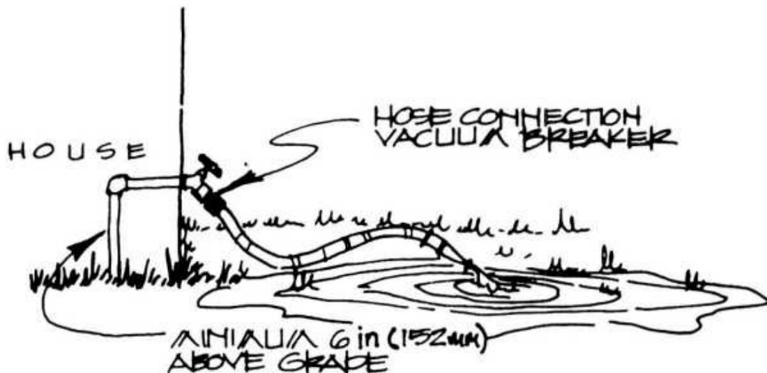
FIGURE 16.7 Hose connection vacuum breaker.
