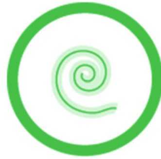
Fig. 15.8 Coil of inline drip tubing around tree
