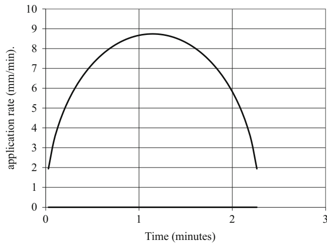
Fig. 12.11 Application rate versus time for point in the field with 2.1 minute application time
