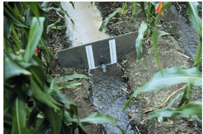
Fig. 20.12 Blocked furrow infiltrometer (Credit NRCS)
