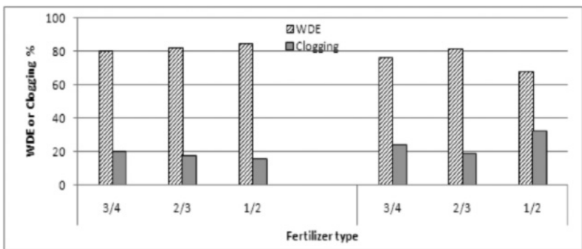
FIGURE 13.2 Effects of fertilizer type and fertigation/ irrigation time ratio on water distribution efficiency (WDE) and clogging.
