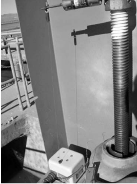
Fig. 2-38. Linear potentiometer and cable used to measure height of sluice gate shaft. These tend to have some temperature-related drift
