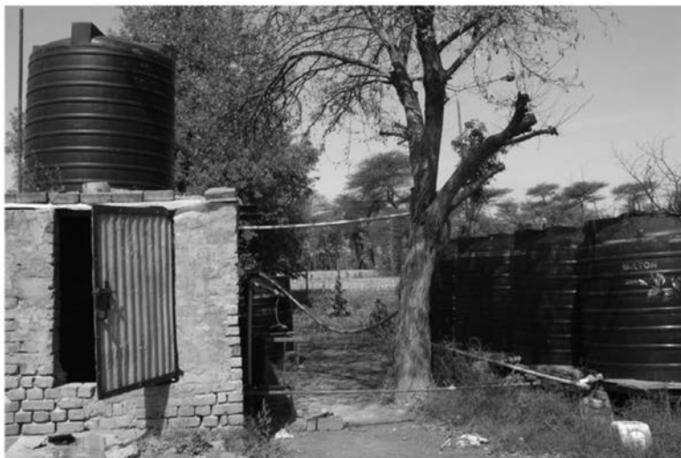
FIGURE 13.4 View of experimental setup for mixing of saline and fresh water.
