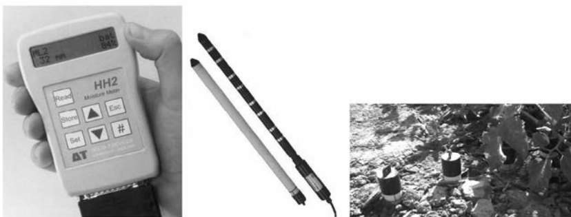
FIGURE 13.8 Delta-T device moisture meter with PR-1 probe; Access tubes fixed in the field near plant for measurement of soil moisture (Extreme right).
