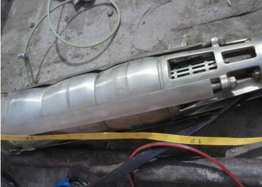
Fig. 15.7 Three Stage Submersible Pump for Solar Tubewell
