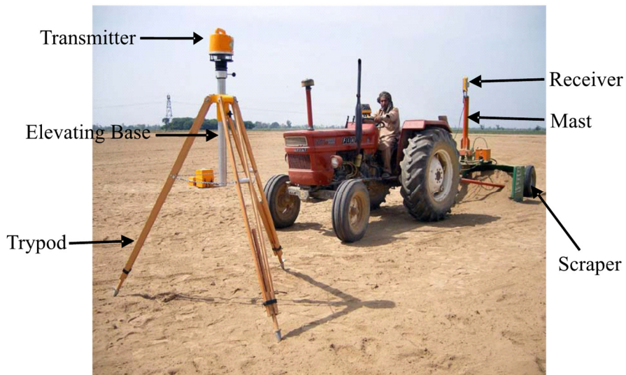
Fig. 9.9 Components of LASER Leveling Equipment
