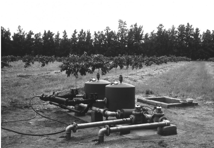
Figure 1.20 Drip irrigation allows the precise application of water to (or below) the soil surface through a network of plastic pipes and emitters. In the foreground, the control-unit connects the network to a water source with valves, filtration and fertiliser injection facilities – Swaziland (MKVC).
