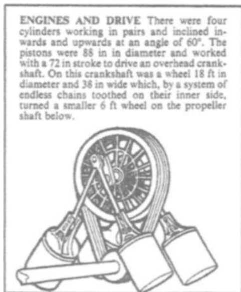
Fig. 1.6—Sketches of the Great Britain propeller shaft fabricated from riveted wrought iron plates and forged wrought iron bearing stubs. The relationship of the four-cylinder steam engine and the chain drive to the propeller shaft is shown also. (Courtesy of The Great Britain Project, Bristol, UK)
