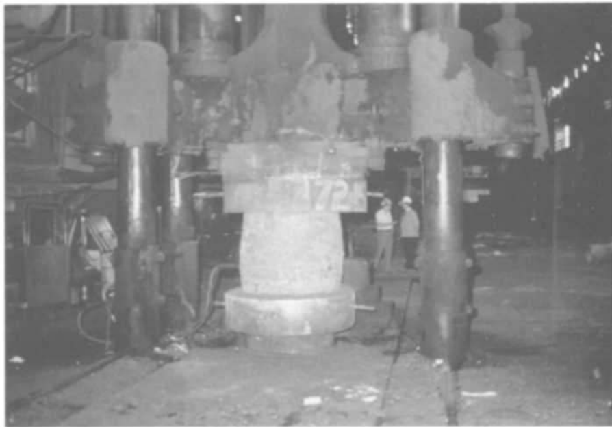
Fig. 5.2 —Stages in the upsetting of a 40-in. (1000-mm) VAR alloy steel ingot. In the top picture the previously prepared tong hold is inserted in the bottom pot die, and in the lower picture, near the end of the upsetting operation the forging has attained the characteristic barrel shape.
