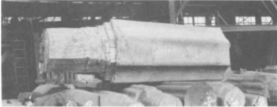
Fig. 2.14 —Alloy steel big end up, octagonal fluted forging ingot with hot top or feeder head. Ingot diameter 42 in. (1050 mm), and weight 44 000 lb (1993 kg). Used to forge one of three sections for the slab forged crankshaft shown in Fig. 2.19.
