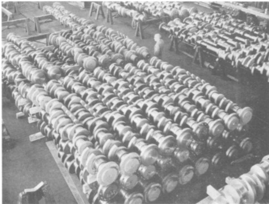
Fig. 2.5 —Continuous grain flow, closed die forged diesel electric locomotive crankshafts. The counterweights were welded to the webs before heat treatment. (Courtesy Ellwood National Crankshaft Company)
