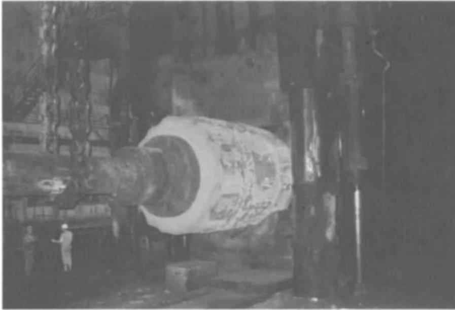
Fig. 5.5 —When the required bore diameter has been obtained by the procedures shown in Fig. 5.4, the forging length can be increased and the OD contoured as necessary by fitting a water cooled tapered mandrel into the bore and forging between the normal transverse top die and a bottom Vee shaped die as illustrated. (Courtesy of The Japan Steel Works, Ltd.)
