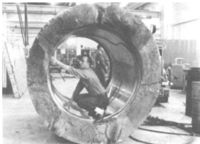
Fig. 9.1 —Brittle failure during hydrostatic testing of a large thick-walled alloy steel pressure vessel for a cold isostatic press. Investigation showed that the principal cause was poor heat treatment that left the forging with a high ductile to brittle transition temperature.
