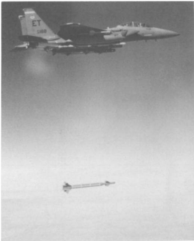
Fig. 19.1—A guided 5000 lb (2265 kg) penetrator warhead being dropped at a test range. The warhead was forged from a high strength low alloy steel with a composition similar to Grade 84 of ASTM A 579/A 579M.
