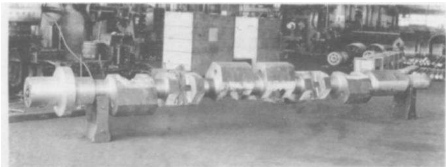
Fig. 2.17 —Crankpins after hot twisting, and drilled prior to sawing excess material from the crankpin locations.
