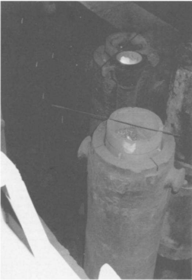
Fig. 4.4 —Thirty-seven-in. (940-mm) VAR electrodes immediately after bottom pouring. The sprue pipe is visible between the molds. The hot tops for the electrodes are topped by the flux that was originally suspended in the molds from the rods lying across the hot tops.
