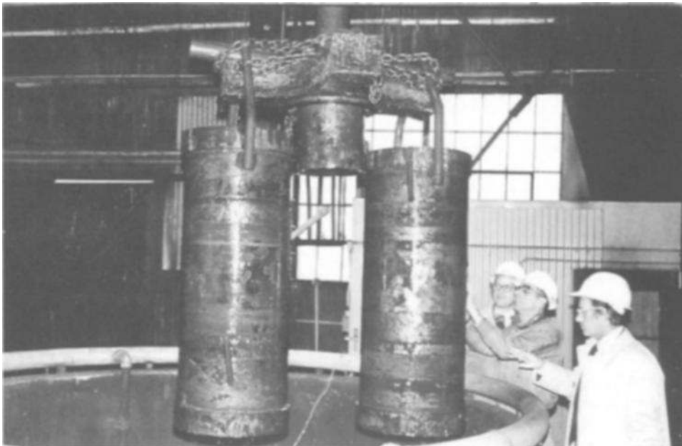
Fig. 9.3—Two pressure vessel shells to ASTM A 508 Class 2 being checked for temperature rise after water quenching. Note the use of type 316 austenitic stainless steel bar as support straps or bales when hanging the forgings in a vertical furnace. Also note the 1-in. (25-mm) tubes tacked to the OD to act as thermocouple pockets.
