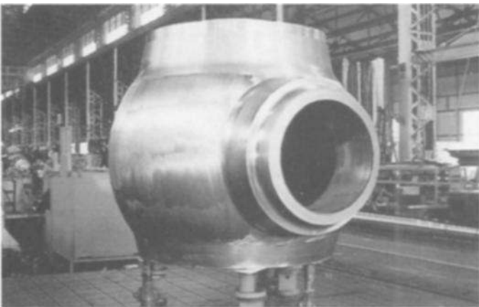
Fig. 2.12 —Forged Boiling Water Reactor (BWR) circulating pump housing to SA-508 Class 3. Outside diameter 96 in. (2400 mm) and 77 in. (1930 mm) high. Weight 16 tons (14.5 t). (Courtesy of The Japan Steel Works, Ltd.)
