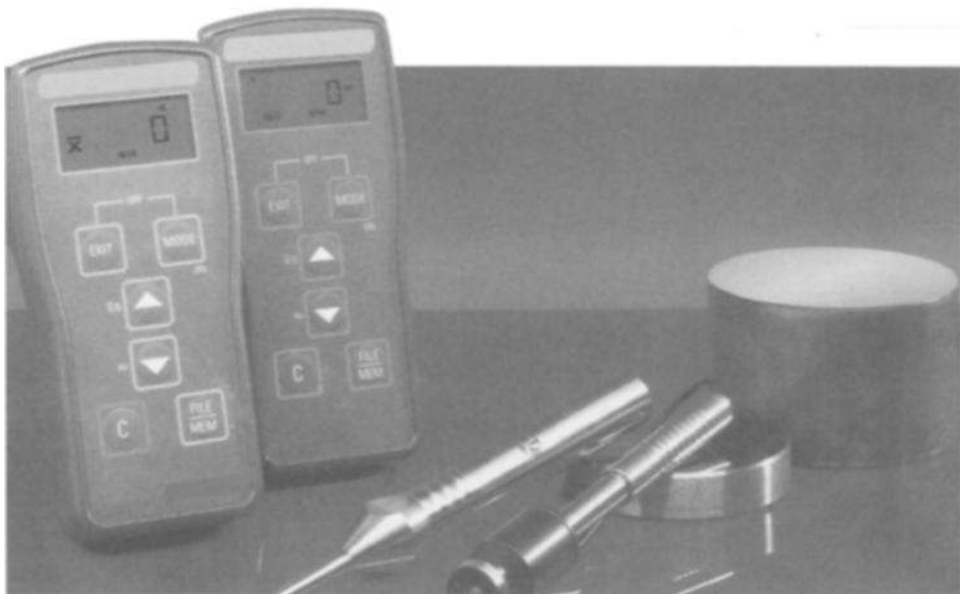
Fig. 16.1 —Examples of commercial Leeb hardness testers. They are typically very portable and normally include built-in conversion to conventional hardness scales as derived by the equipment manufacturer. Note the thickness of the hardness test block in the lower picture. (Courtesy of Proceq SA (top) and GE Inspection Technologies (bottom))
