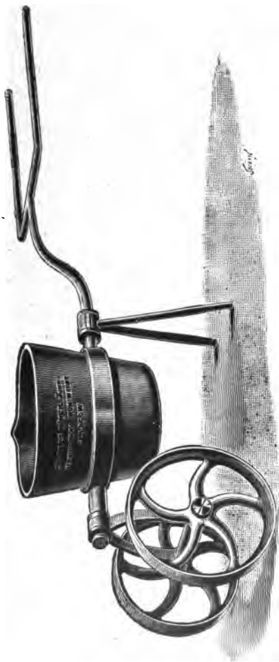
Fig. 70.—Moulder's Ladle Mounted on Wheels.
