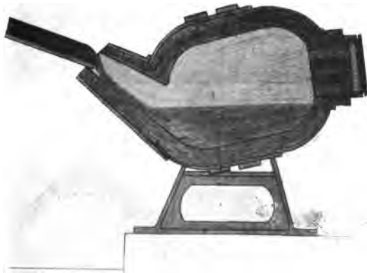
Fig. 29.—Pouring "Metal" into a Converter.
