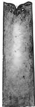
Fig. 55. — Sketch representing Vertical Section of Partly-cooled Ingot.
