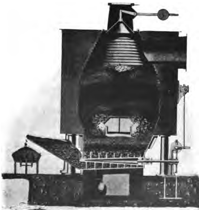
Fig. 38.—Wilson Gas Producer with Archimedian Screw for removing ashes.
