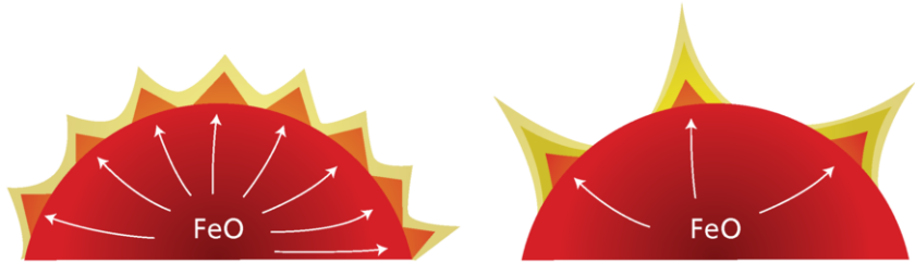
Figure 3.8 Balance between iron nucleation and nuclei growth. Limited swelling accompanied by the formation of an iron shell (left). Limited iron nucleation followed by strong needle growth of the nuclei with as a result excessive swelling of the pellet (right).
