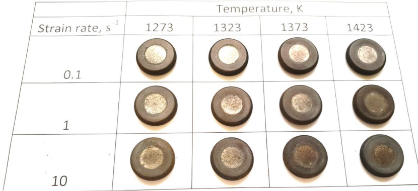
Figure 3. The images of the samples after hot deformation.
