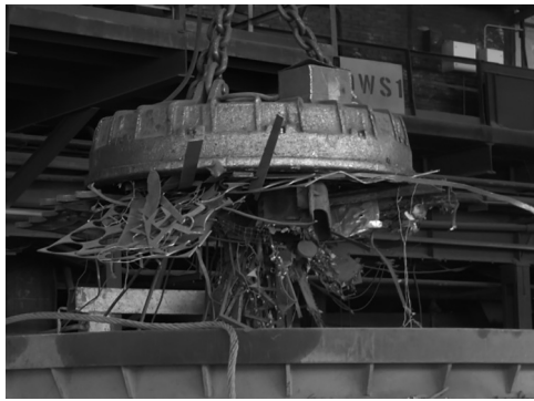
FIGURE 9.5 View of an electromagnetic gripper with suspended scrap. (Author's photo.)
