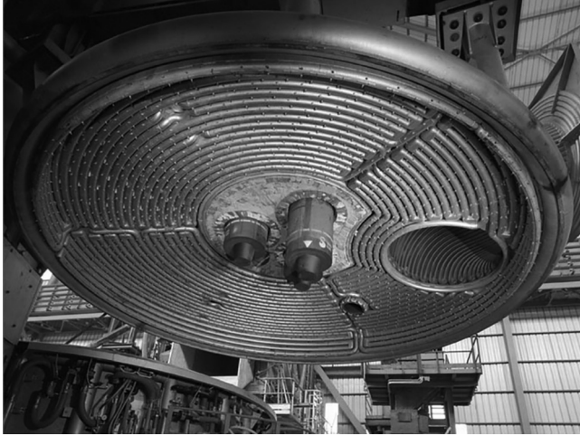
FIGURE 3.40 The bottom view of the water-cooled roof for a smaller size electric arc furnace, tubular panel type, with a round central part [17]. (Advertising materials (corporate brochure) of the SMS group GmbH (formerly Mannesmann Demag Huttentechnik SMS Siemag AG) – with permission.)
