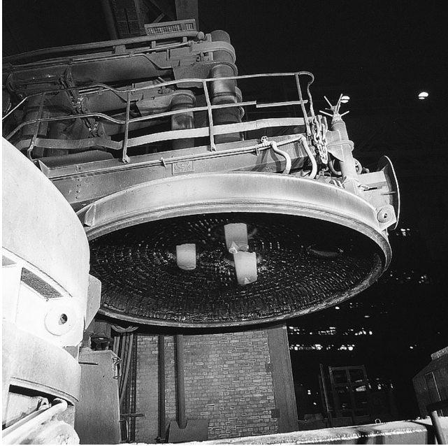
FIGURE 3.39 The bottom view of a water-cooled roof after swinging from the operating electric arc furnace [17]. (Advertising materials (corporate brochure) of the SMS group GmbH (formerly Mannesmann Demag Huttentechnik SMS Siemag AG) – with permission.)
