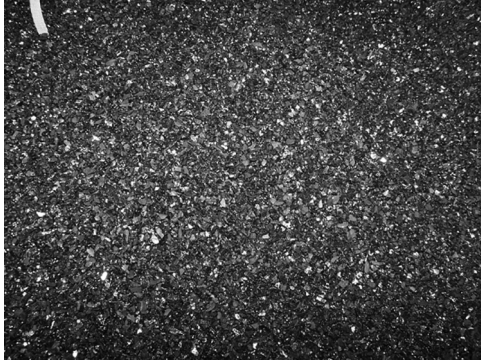
FIGURE 8.11 View of anthracite carburizing agent with a grain size from 1 to 3 mm. (Author's photo.)
