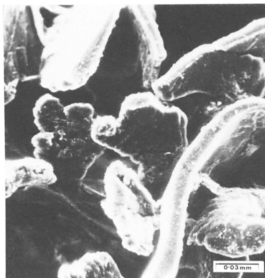
Figure 6.11 shows an S.E.M. micrograph of a compacted iron made by using a Mg–Ce–Ti addition to control the graphite morphology. Compared to Figure 6.9 the flakes are thicker and the edges are blunt. In common with Figure 6.9 the flakes are interconnected. (Courtesy BCIRA).
