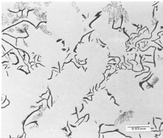
Figure 6.41 shows the structure of Nicrosil austenitic cast iron of composition
