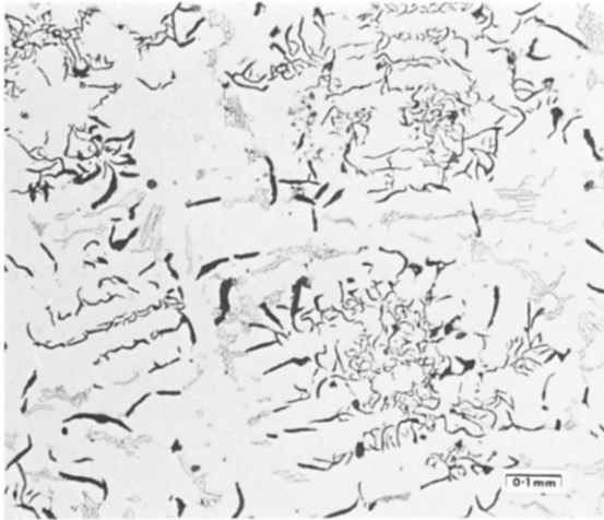
Figure 6.39 shows the structure of a Ni-resist austenitic cast iron of composition
