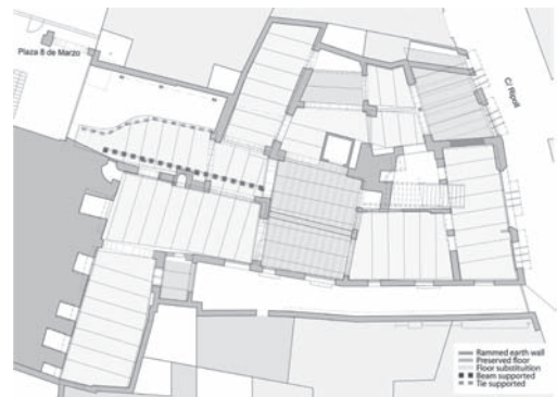
Figure 8. Location of rammed earth walls in the main (first) floor. Picture: S. Bestraten–E. Hormias.
