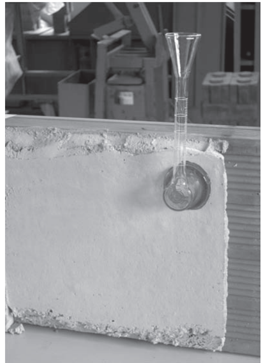
Figure 2. Water capillary absorption tests.
