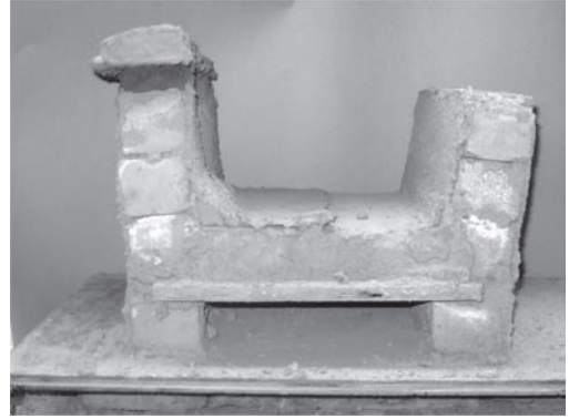
Figure 9. The reduced scale model and the sacrificial layer on the top of the parapets.
