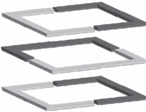
Figure 3. Building system used alternating the available U-shaped formwork (Vegas & Mileto).
