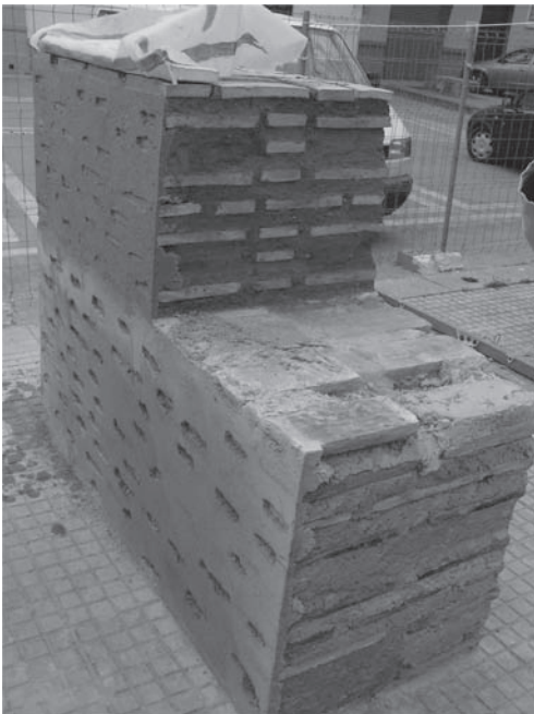
Figure 8. Tests carried out to build the valencian rammed-earth wall.
