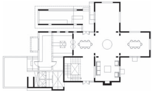
Figure 9. Plan of the admin block of Forsyth Lodge, Building 5. The shaded walls are the rammed earth walls.
