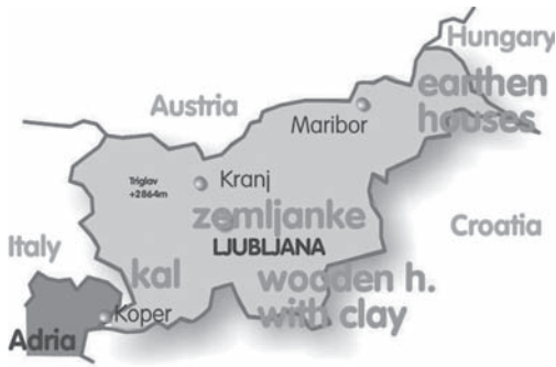
Figure 4. Slovenia and use of clay: in the Karst region it enables the ponds, in the central region it is cut for storing rooms, in the Eastern part it is used in cob and rammed houses, in the South it serves as filling in the wooden constructions.
