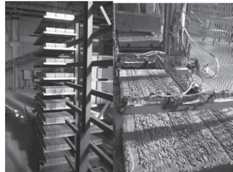
Figure 5. The industrialized adobe production line (photo: M. Brioni).
