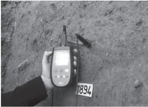
Figure 5. Temperature measurement of pottery fragments embedded in a rammed-earth wall.
