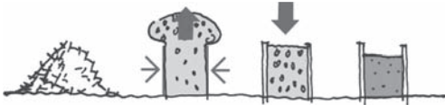
Figure 2. Clay in chips has to be squeezed to expel the air. Density of the clay is so higher, and material becomes more constructive.
