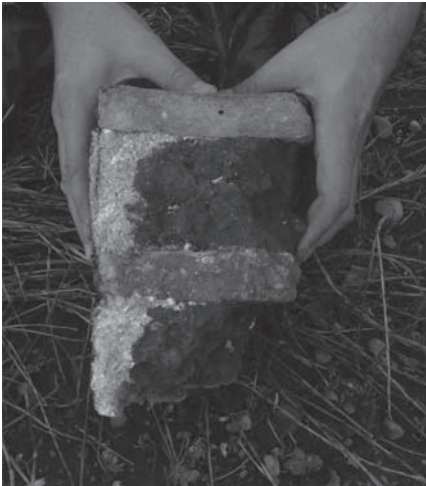
Figure 2. Mortar core, ceramic connectors and crust. Three detached parts of a tapia valenciana wall. (Authors: Cristini & Ruiz Checa).
