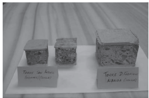
Figure 4. Photographs of three cubic wall cores capped with sulfur.
