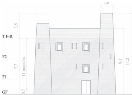
Figure 5. Elevation of the tighremt shown in Figure 4. Height is given in meters and in number of wall sections.
