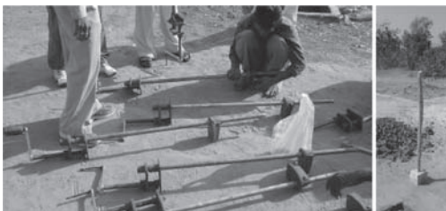
Figure 11. Clamps used in the formwork and wooden rammer, fabricated locally.
