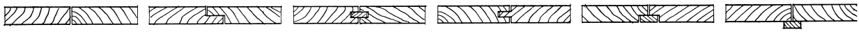
butt joint 'tsugi-tsuke' shiplap joint 'wajaku-ri' spline joint 'yatoi-sane' tongue/groove 'hon-sane' batten joint 'shiki-me' batten joint 'enke'
