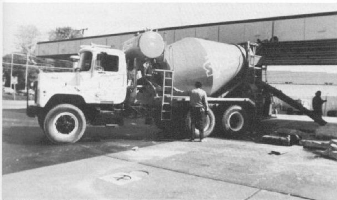
Fig. 4-6. A typical barrel type of concrete truck.
