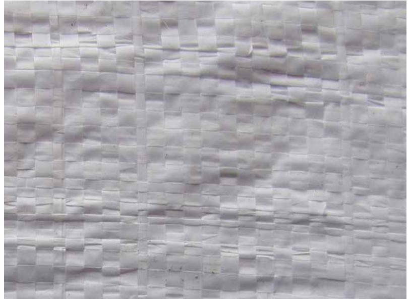
Fig. 4.1: This close-up of a polypropylene bag shows the woven nature of the ribbons of the poly material, which allows for some breathability.
