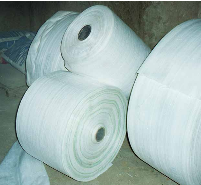
Fig. 4.3: These rolls of polypropylene tubing are ready to be cut to lengths appropriate for building. CREDIT: KELLY HART
