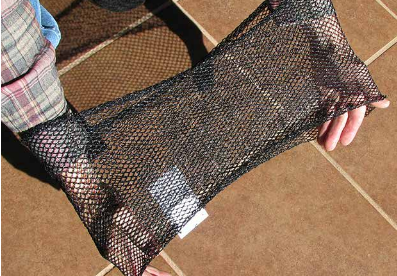
Fig. 4.2: This open raschel mesh tubing can be used with the Hyperadobe method. CREDIT: ROSANA HART
