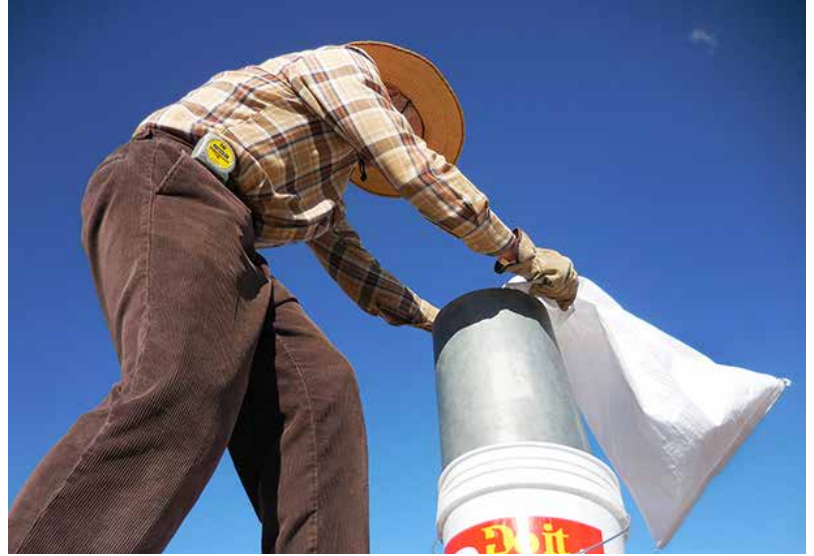
Fig. 5.1: Here the author is about to slip a new bag over the narrow end of a chute that was originally the upper part of a commercial chicken feeder.
