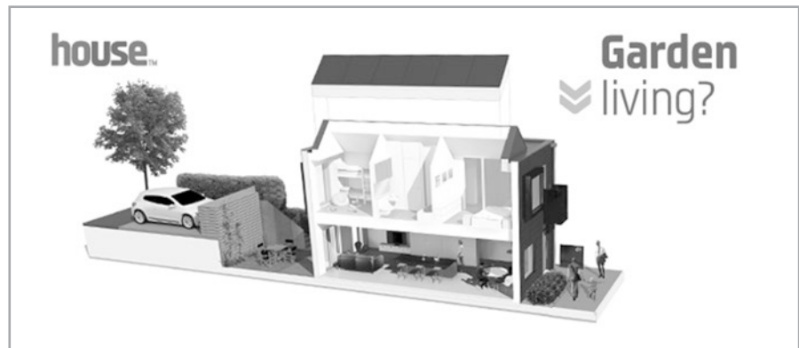
Figure 7.72 Cross section through the Urbansplash 'HoUSE' volumetric dwelling. (image with kind permission of Urbansplash)
