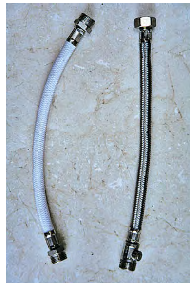
Connecting the pipework to the taps can be a bit 'fiddly'. Flexible connectors (the right-hand one with an integral isolation valve) make things a little easier.
