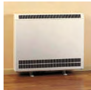
Modern storage radiators can respond to changes in external temperature when charging, and respond to varying temperatures during the day. Some of them are fan assisted.
