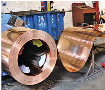
Most cylinders are still handmade out of copper sheet.
