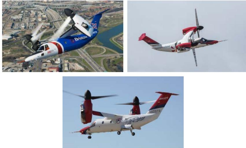
**Fig. 10.5** The AW609 tiltrotor in conversion mode (top left) and helicopter mode (bottom) (photos Leonardo Helicopters) and in airplane mode (top right) (photo courtesy Jay Miller – AHS International)
