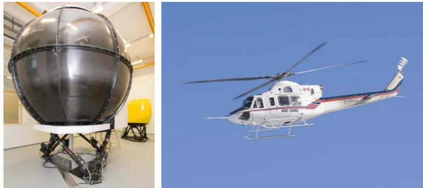
Fig. 3.49 The UoL HELIFLIGHT-R ground-based flight simulator (left) and NRC ASRA in-flight simulator (right) (Ref. 3.92)
