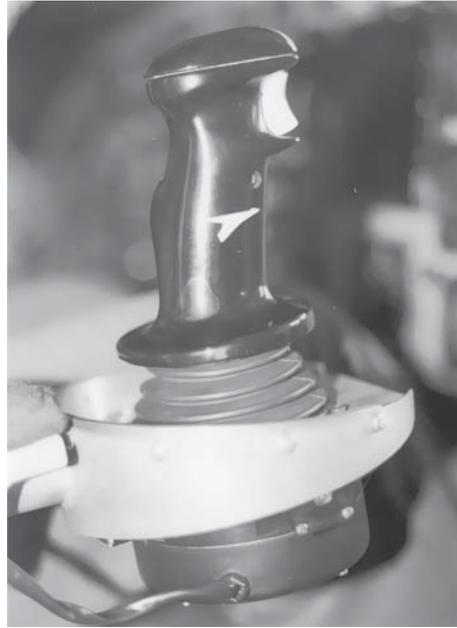
**Fig. 2.48** CAE four-axis sidestick onboard the Canadian NRC variable stability Bell 205
