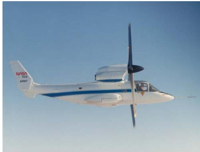
**Fig. 10.2** The XV-15 tiltrotor in airplane mode (NASA)
