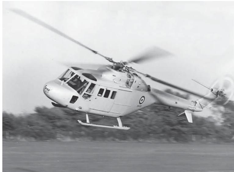
**Fig. 9.14** Prototype Lynx with experimental underfins to improve yaw stability.
