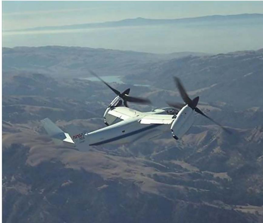
*The XV-15 research aircraft, designed and built by Bell Helicopters, first flew on 3 May 1977 and was operated by NASA and the US Army, delivering proof of concept demonstrations and multiple research outputs over more than 25 years. Results from research using simulations of this aircraft, undertaken by the author and colleagues, feature throughout this chapter. Source: Photo NASA*
