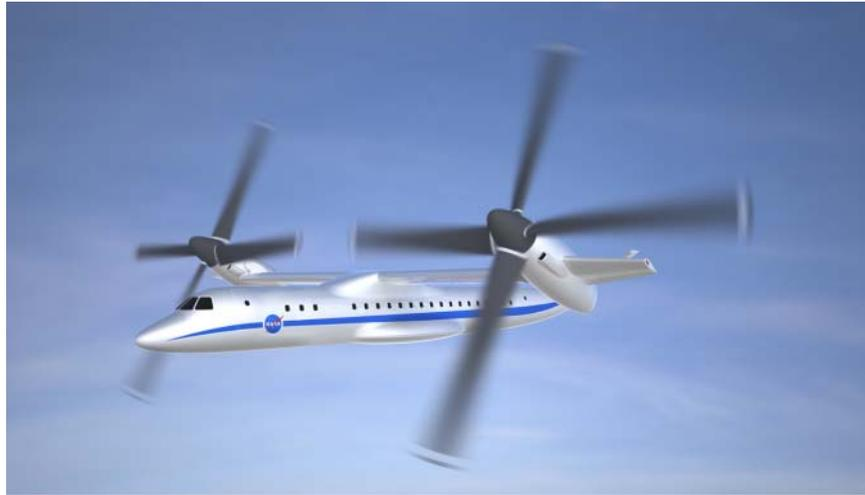
**Fig. 10.80** Artist's impression of NASA's Large Civil Tiltrotor2 (LCTR, second generation, image NASA)
