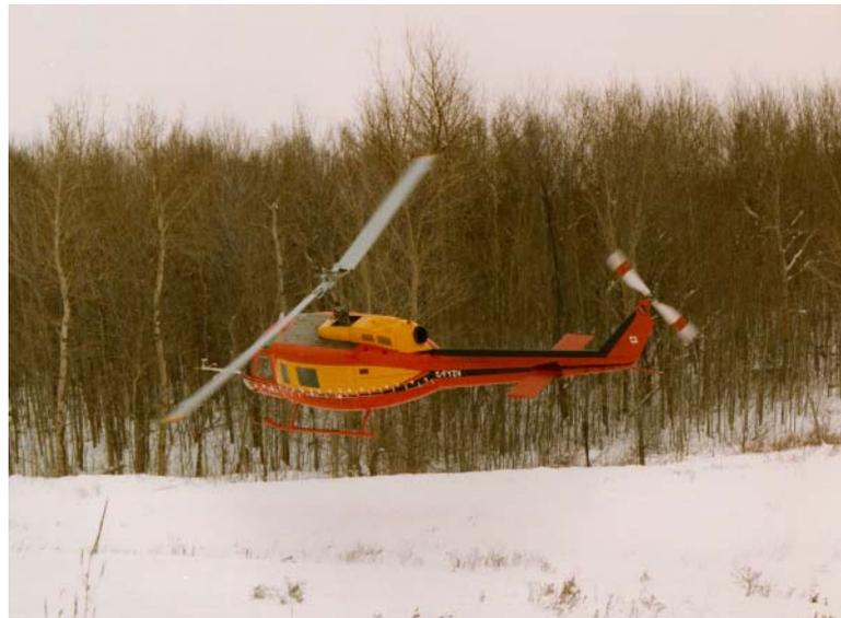
Fig. 9.22 The Bell 205 in-flight simulator operated by the NRC Flight Research Laboratory. Source: From the author's collection
