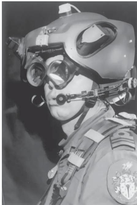
**Fig. 2.49** GEC biocular helmet-mounted display
