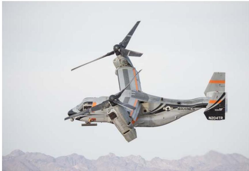
**Fig. 10.7** The Bell-Boeing V-22 Osprey tiltrotor in conversion mode (photo courtesy Jay Miller – AHS International; showing Bell’s experimental V-22 testbed)
