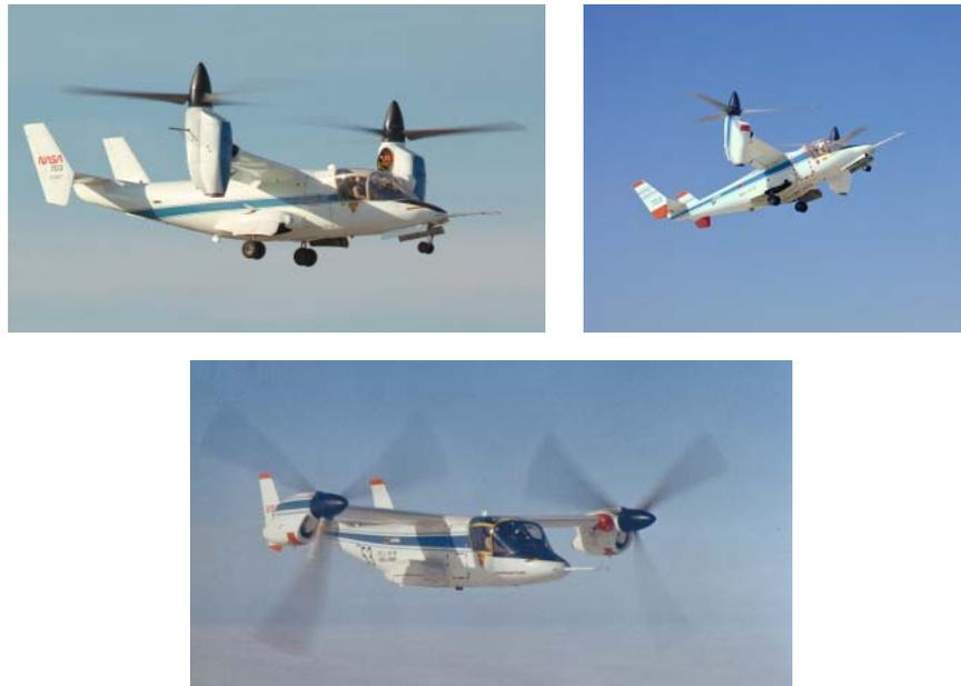
Fig. 10B.1 The XV-15 in helicopter, conversion and airplane modes (NASA)
