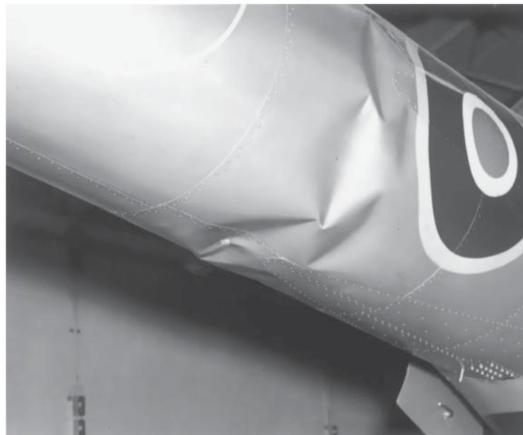
**Fig. 2.38** Fuselage failure on Sikorsky S-51 (Ref. 2.31)
