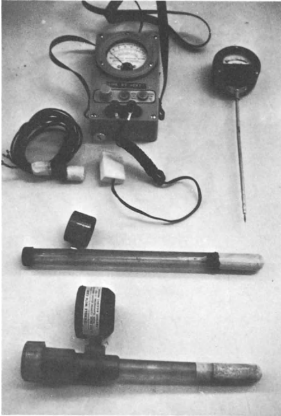
Fig. 5-26. Common devices for estimating soil moisture content. Two devices in lower part of photograph are porous, clay cup tensiometers, adequate to suctions of about 800 cm water: Electrical device in upper part, with two styles of plaster blocks is a Bouyoucos bridge, suitable for suctions in excess of 1 bar. Narrow probe on right is another electrical device seldom seen in practice, due to the fact that soluble salts greatly influence its reading
