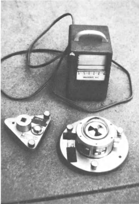
Fig.2-32. Two types of radiometric sensors for measuring radiation between 3 and 3000 nm, together with an inexpensive recording device for measuring output from the silicon cell ( left ). The glass-covered sensor ( right ) is an Eppley pyranometer, standard U.S. Weather Bureau radiometer for measuring short-wave solar radiation
