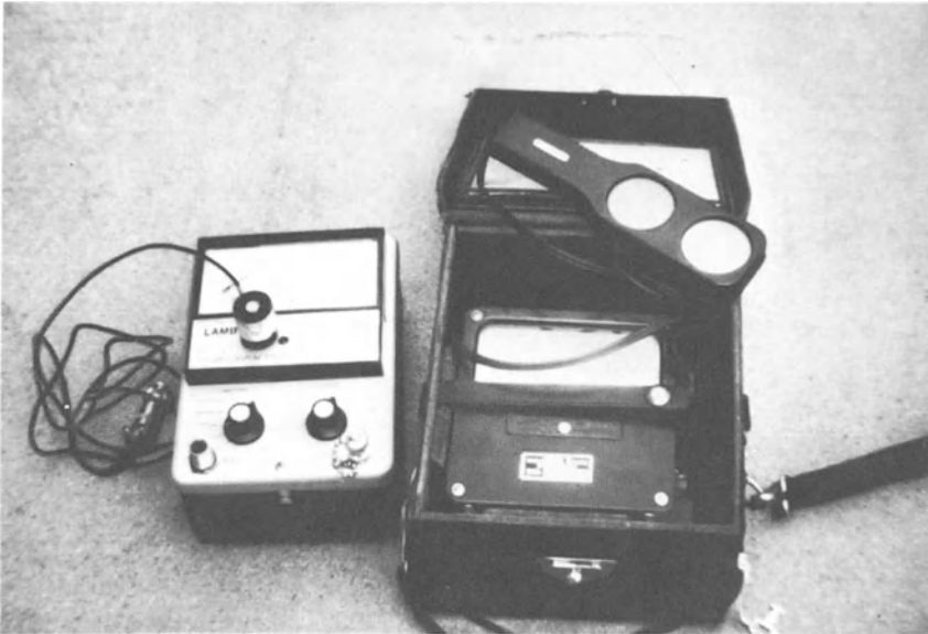
Fig. 2-31. Two types of photometric sensors. Left : “Lambda meter”, evaluates in lux and is cosine corrected. Sensors are interchangeable to measure photosynthetically active radiation in “Einsteins” or total radiation in gm\text{-}cal\text{ cm}^{-2} . Right : “Illuminometer”, with output in foot-candles, noncosine corrected, but color-corrected for human eye sensitivity. Latter usable only for direct radiation, perpendicular to receiving surface, and is most common type employed in the U.S.
