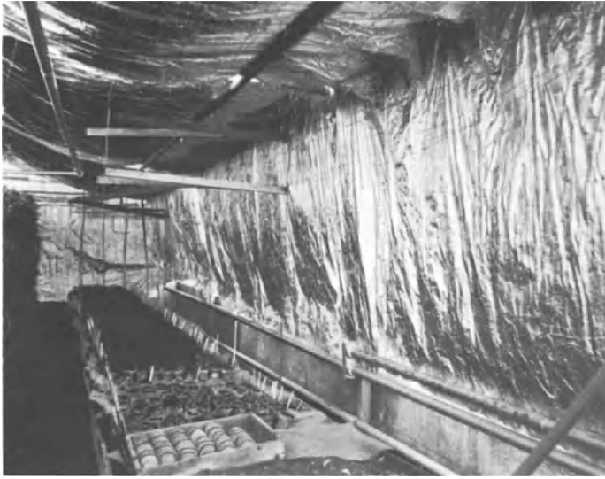
Fig.4-37. Aluminum lined heat blanket in position for heat conservation studies (Tristan, 1975)
