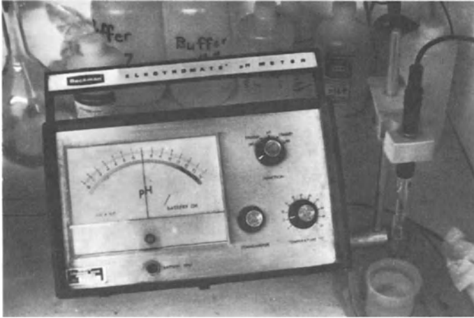
Fig. 7-13. pH meter for determining the acidity or alkalinity of an extracted solution from a soil sample. Right : measuring electrode
