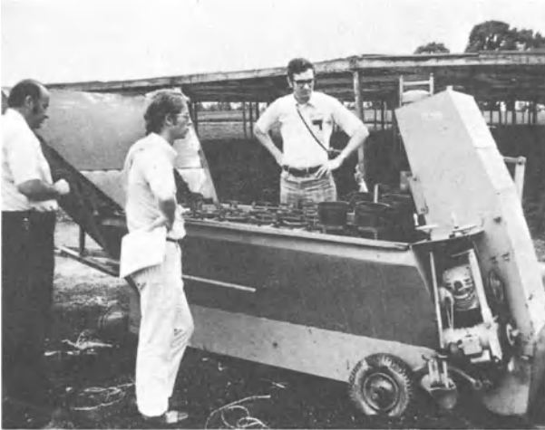
Fig.6-14. Potting machine. Soil is loaded on left. Workers set pots on conveyor which passes them under loader at right. Such machines will fill more than a thousand pots per hour. A large crew will be required if machine is to be maximally utilized
