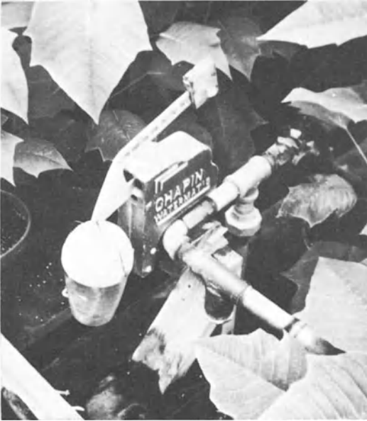
Fig. 5-37. One type of irrigation timer for pot watering. Watering cycle must be initiated by operator, but shuts off automatically when weight of water in cup exceeds a preset limit. (Courtesy of J.W. White, Penn. State Univ.).
