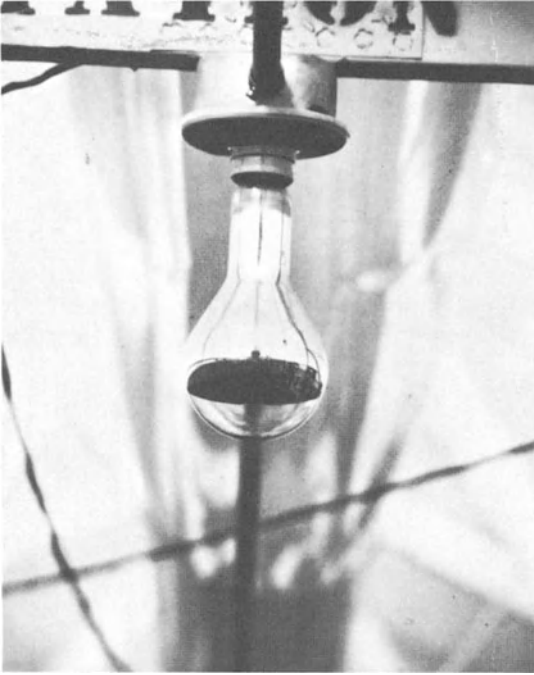
Fig.2-28. 200-W bulb with internal reflector commercially employed for photoperiodic control
