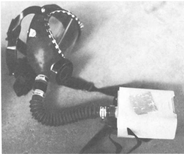
Fig.9-22. Gas mask with a filter suitable for most organophosphates. Efficacy of gas masks will depend upon their proper maintenance and cartridge replacement
