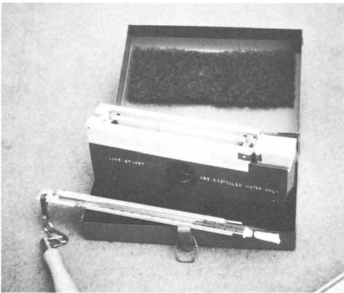
Fig. 5-9. Two types of psychrometers for measuring relative humidity. To achieve adequate ventilation, lower psychrometer is whirled. Cased psychrometer contains battery-powered fan to achieve ventilation, and is less susceptible to breakage
