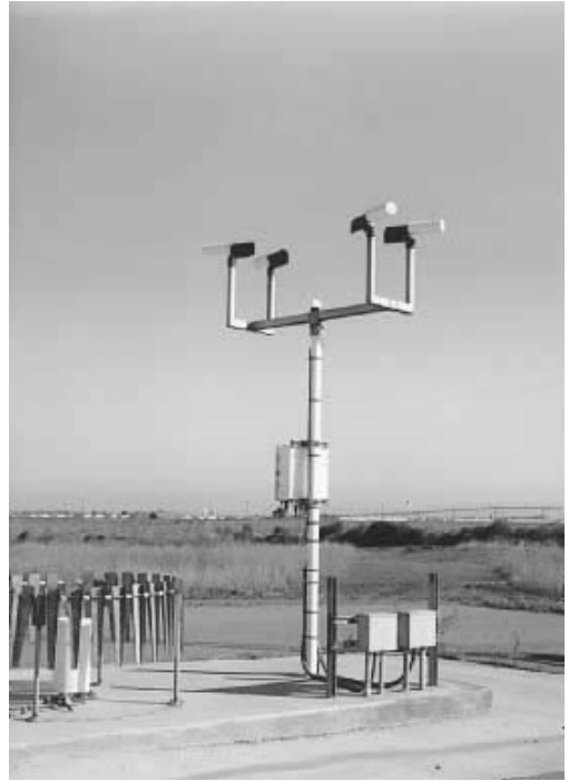
Fig. 1-4. A scatter meter device indirectly measures how far one can see.
