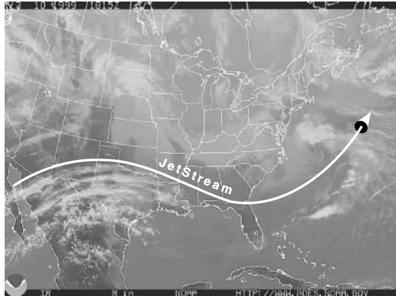
Fig. 3-6. Recall that on IR images high clouds are cold and bright, low clouds warm and gray.
