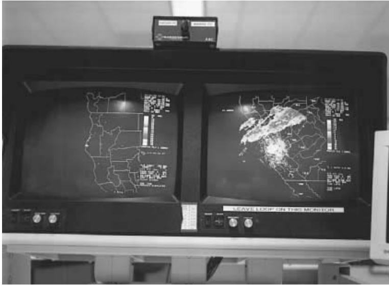
Fig. 9-2. The NEXRAD radar provides the radar specialist with a computer display of radar echoes, including the relative motion within a storm system.
