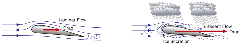
Figure 4-36 Ice accretion on the airframe will increase drag.
