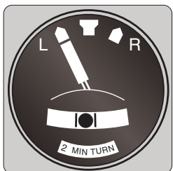
Figure 10-26 The modern turn coordinator (top), and the older turn indicator, each indicating standard-rate turns to the left.
