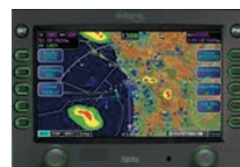
Figure 16-25 Combined weather radar ground map display.
