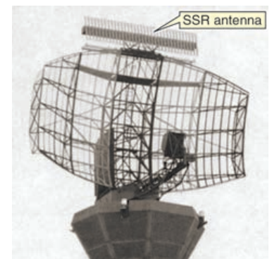
Figure 16-17 SSR antenna on top of radar head.
