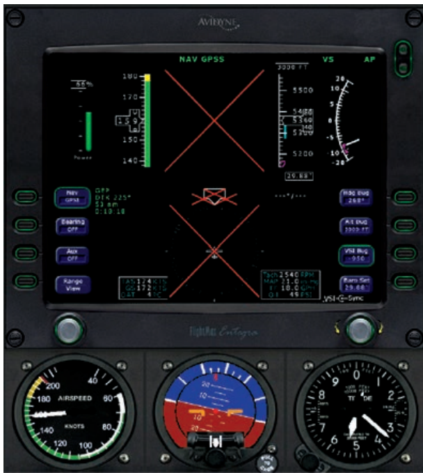
Figure 29-22 PFD with AHRS failure indications.
