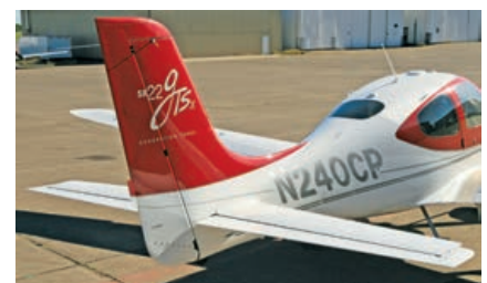
Figure 4-7 Vertical stabilizer and rudder.
