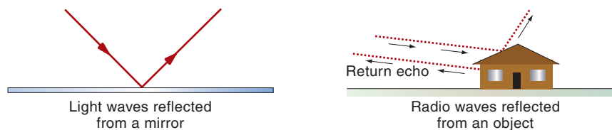
Figure 16-6 Some radio waves can be reflected in a similar way to the light waves.
