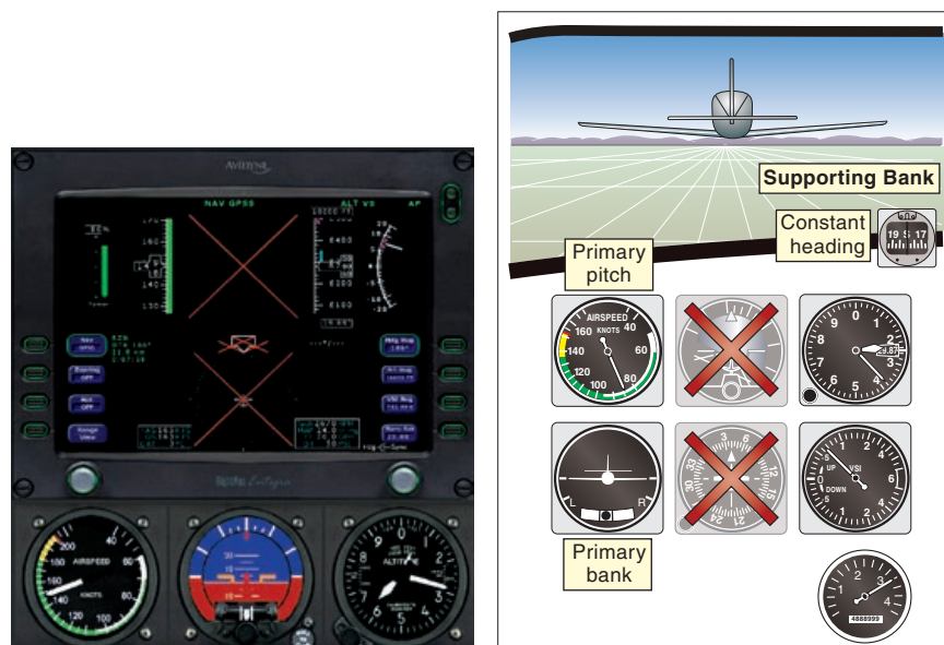
Figure 29-13 Maintaining the climb on a partial panel.
