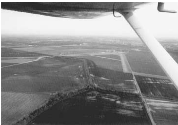
Fig. 5-6 This pilot has waited too long to turn from base leg to final approach, a very common error. This is a prime area for an approach-to-landing stall.
