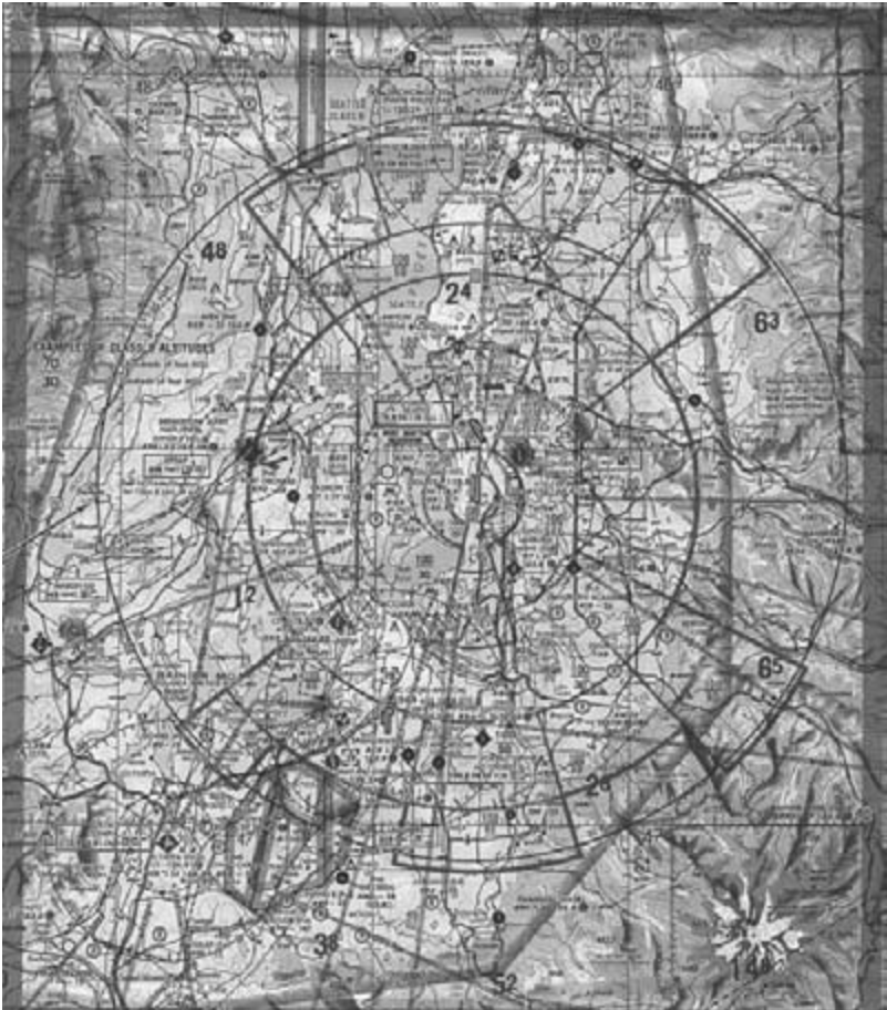
Fig. 20-8. The large band-box helps identify a Class B airspace and also represents the area covered by the exploded and more detailed terminal area chart (TAC).
