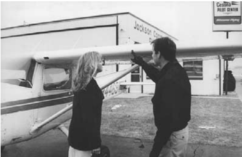
Fig. 1-6 The wing should be checked for any obvious problems such as dents, loose rivets, blocked pitot tube, etc...
