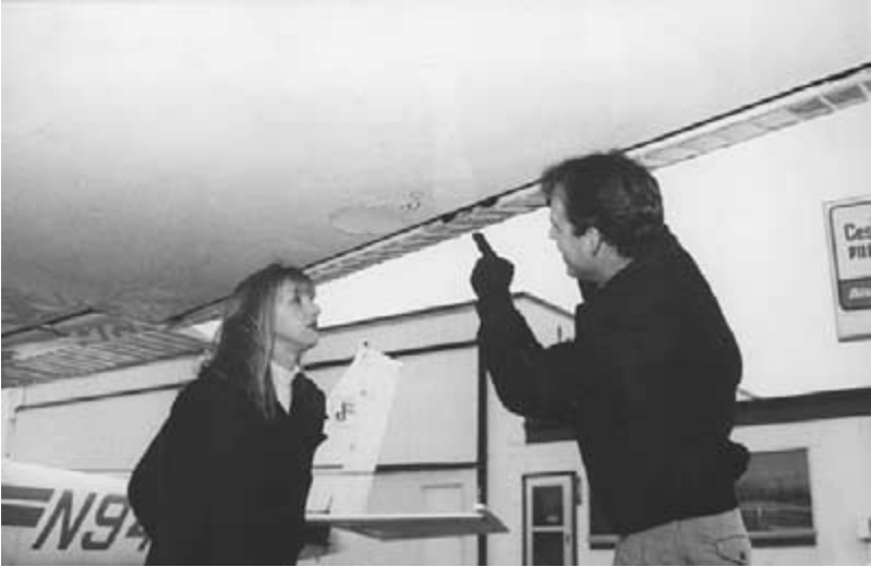
Fig. 1-7 When you check the actuating rods of the ailerons, hold the aileron in the up position so a sudden gust of wind doesn't shorten your finger.
