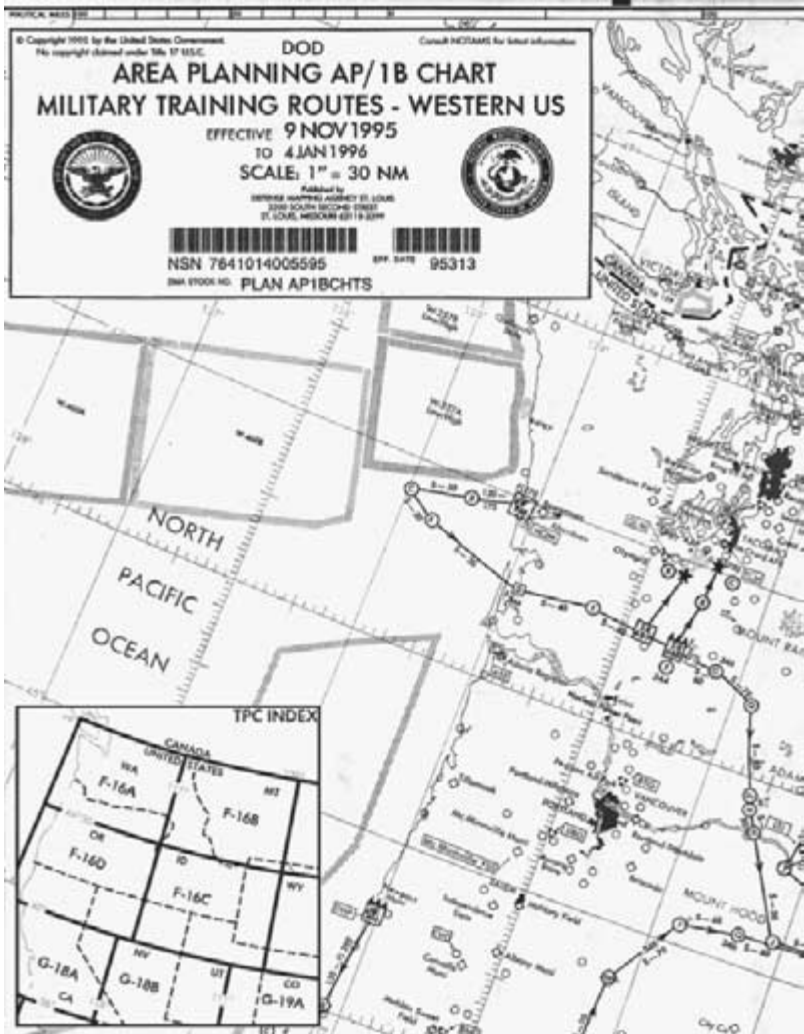
Fig. 13-5. Military training route charts provide a detailed, visual depiction of low-level high-speed routes.
