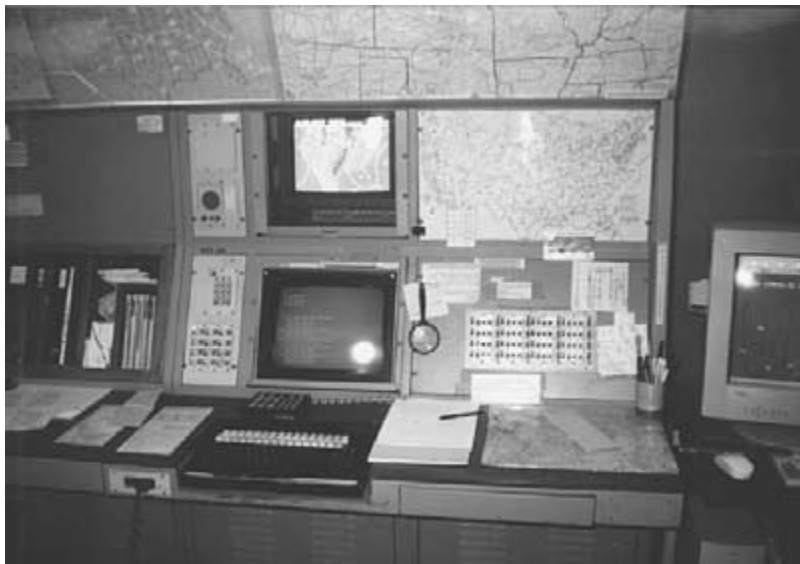
Fig. 26-5. The flight watch position is equipped with charts, video images, and related data to help the specialist provide in-flight pilots with the most up-to-date weather reports.
