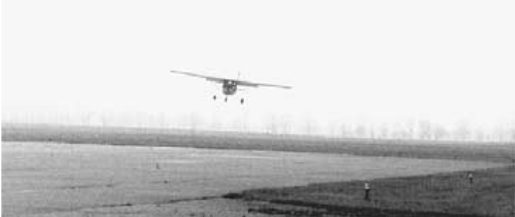
Fig. 5-11 Crosswind landing approach. Wing down into the wind with enough rudder to hold the aircraft straight down the runway.
