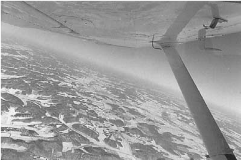
Fig. 3-21 Left view, just prior to stall. The airplane is moving parallel with the horizon—note the angle of attack.
