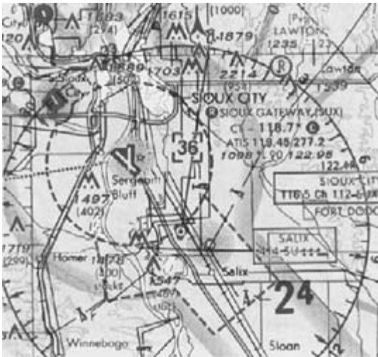
Fig. 17-9. A star to the immediate right of the tower frequency and just before CTAF symbol identifies the tower as part-time.
