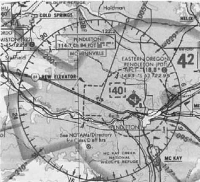
Fig. 17-14. This Pendleton, Oregon, excerpt from the Seattle sectional shows how a Class D airspace extension—the keyholelike design to the west of the airport symbol—is charted.
