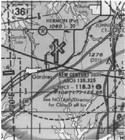
Fig. 20-1. The “NFCT” located to the left of the tower frequency identifies that tower as nonfederal and thus operated by private contractors.
