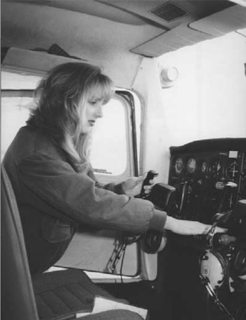
Fig. 1-4 The interior preflight consists of checking the paperwork, fuel quantity, fuel selector, mixture, flaps down, throttle idle, master and mags OFF.
