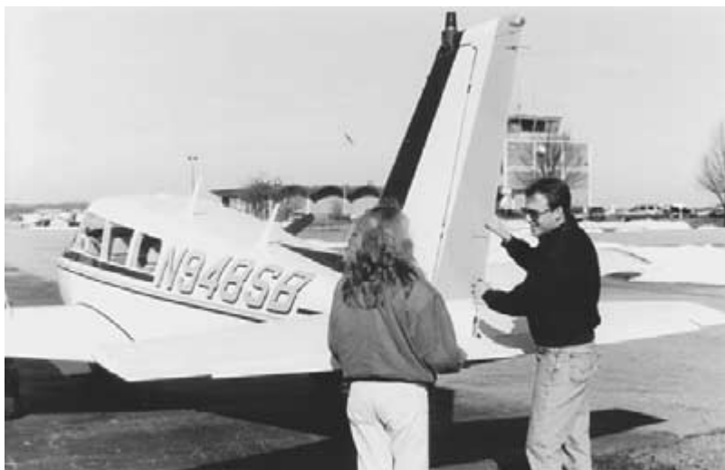
Fig. 8-6 The rudder trim saves a lot of legwork when flying with one engine out.
