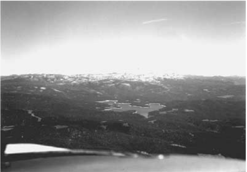
Fig. 12-21. Be careful about using lakes as checkpoints when many similar lakes are in the same general area.
