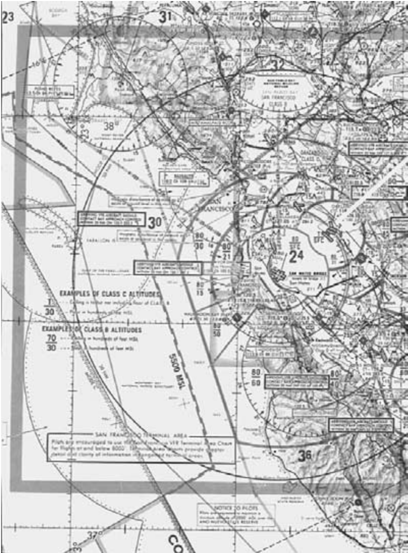
Fig. 12-12. The sectional is satisfactory for operating outside of Class B airspace, but operations close to or underneath Class B airspace require the appropriate terminal area chart.
