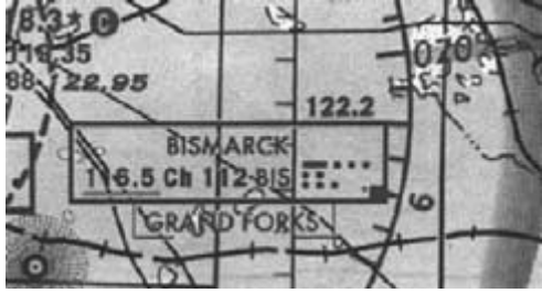
Fig. 26-9. The small square in the lower right corner identifies the VORs that transmit HIWAS.
