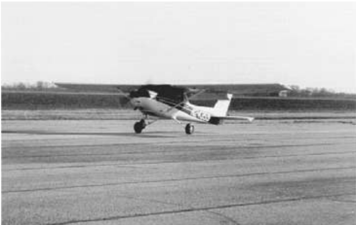
Fig. 5-7 A normal landing with full stall, full flaps, and full back stick.
