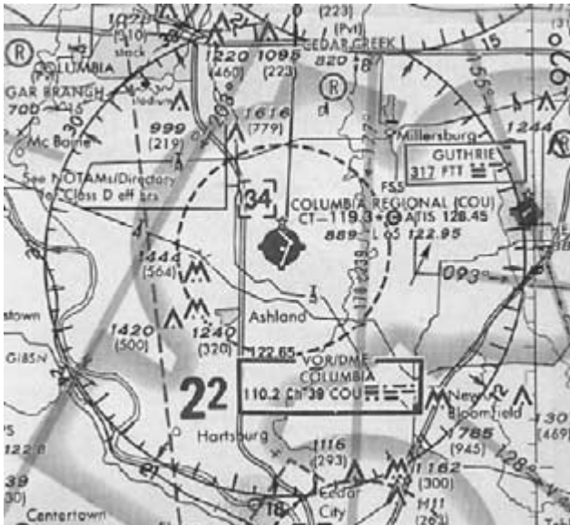
Fig. 24-2. Columbia Regional is an example of a tower-controlled airport with a unicom facility for nonoperational services.
