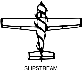
Fig. 3-8 Spiral slipstream creates lift across the vertical stabilizer, which swings the nose to the left.
