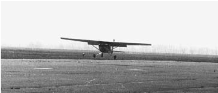
Fig. 5-12 Just prior to touchdown in a left crosswind. Wing is still down and rudder is used as needed to maintain alignment with the runway.
