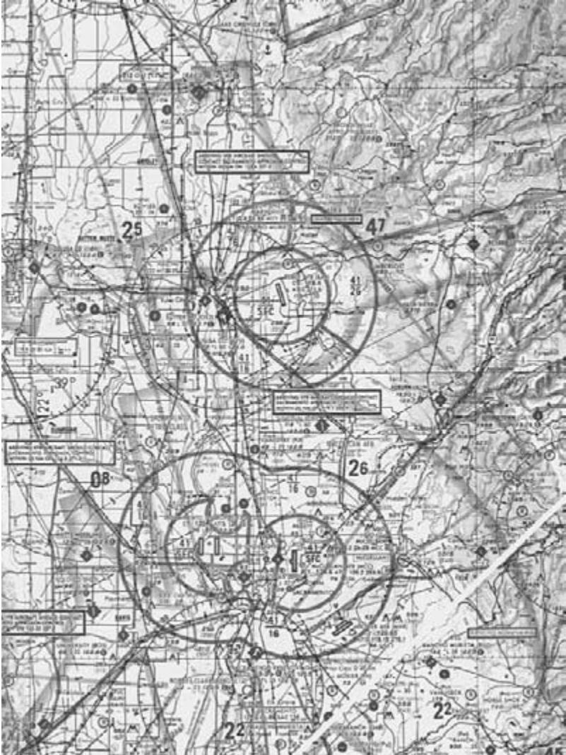
Fig. 12-13. A sectional is required for operating into or in the vicinity of Class C airspace.
