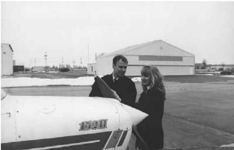
Fig. 1-5 Always check the prop for any signs of nicks or cracks.
