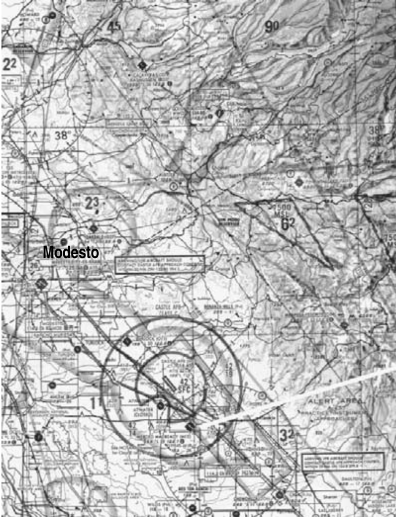
Fig. 11-1. Chart relief is represented by contour lines, shaded relief, and color tints.
