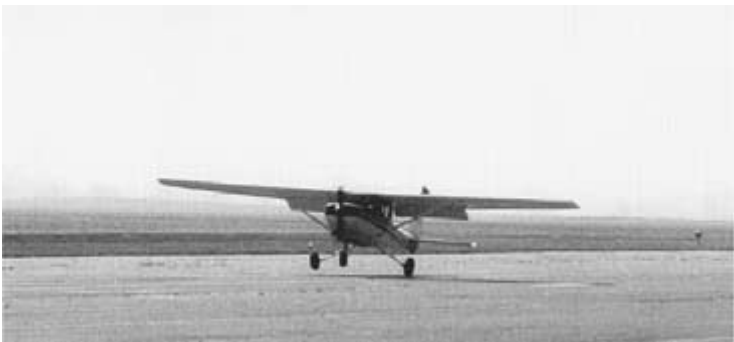
Fig. 5-13 Crosswind touchdown. Upwind wing down, rudder as required to maintain alignment; upwind wheel touches first.
