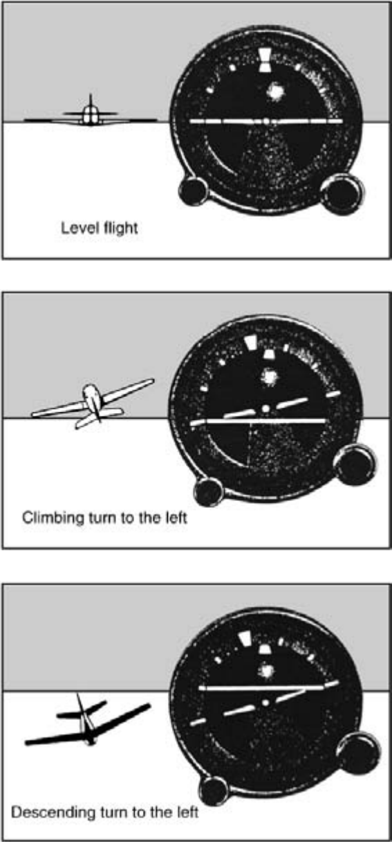
Fig. 3-2 Attitude indicator or “artificial horizon” showing level and turns both right and left.
