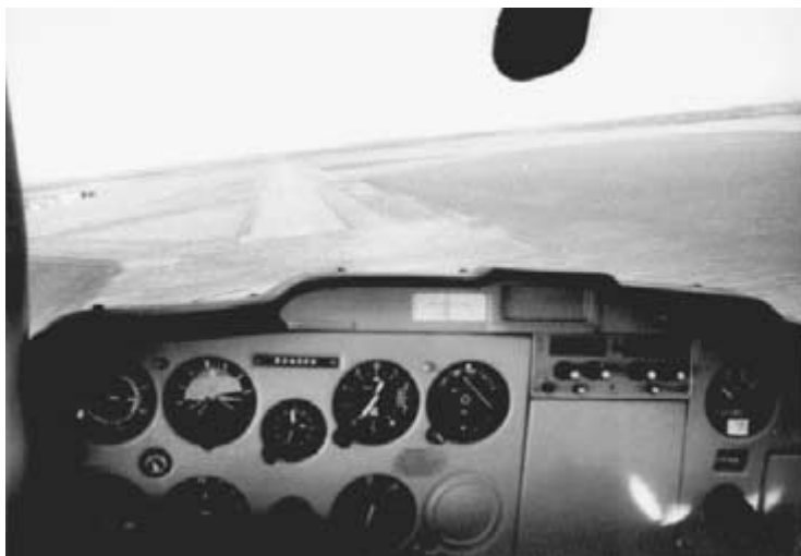
Fig. 5-10 A sideslip as viewed from the cockpit. The wing is still down into the wind, but the aircraft is now aligned with its longitudinal axis parallel to the runway. This is the correct way to land in a crosswind from the right.
