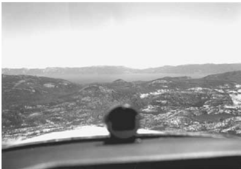
Fig. 12-22. The airplane is above the crest of the mountains because the terrain behind appears to be descending in relation to the crest.
