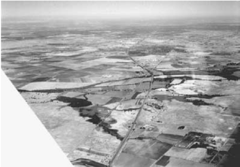
Fig. 12-18. Locating the point where a road and railroad cross can fix the aircraft's position.
