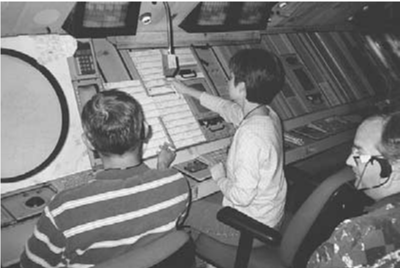
Fig. 22-6. A typical controller's position in a Center, with the PVD and the flight strip racks.
