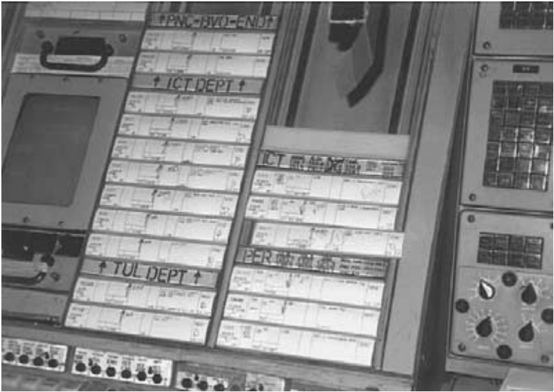
Fig. 22-7. The IFR flight strips for yet-to-depart aircraft are on the left. Those en route are on the right.
