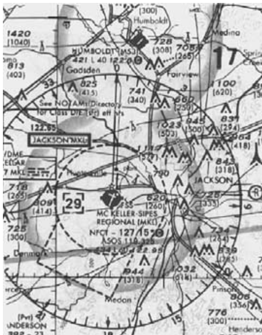
Fig. 17-15. A Class E extension (southwest of the airport) to a Class D airspace is illustrated in this McKeller-Sipes (Tennessee) airport. Note that the Class D segmented circle is closed and the Class E extension is added on, whereas in Fig. 17-14, the circle is not closed and the entire area within the segmented design is Class D airspace.
