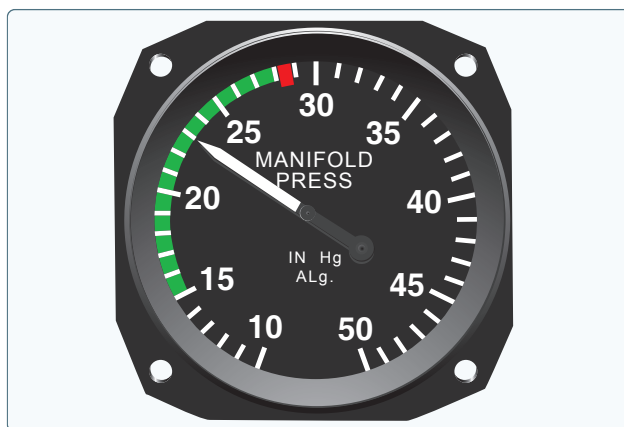
Figure 7-9. Engine power output is indicated on the manifold pressure gauge.
