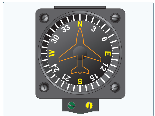
Figure 8-38. Vertical card magnetic compass.
