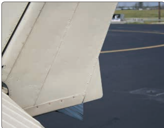
Figure 6-22. A ground adjustable tab is used on the rudder of many small airplanes to correct for a tendency to fly with the fuselage slightly misaligned with the relative wind.
