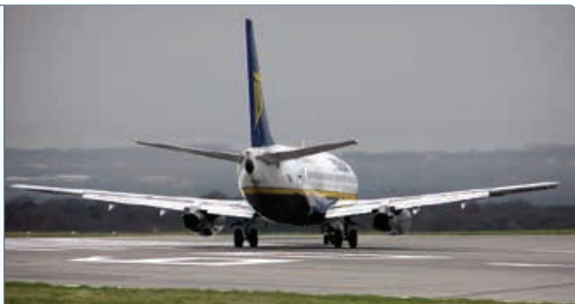
Figure 5-28. Dihedral is the upward angle of the wings from a horizontal (front/rear view) axis of the plane as shown in the graphic depiction and the rear view of a Ryanair Boeing 737.
