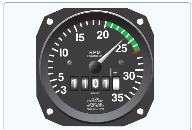
Figure 7-8. Engine rpm is indicated on the tachometer.
