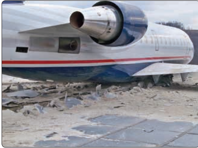
Figure 14-57. There have been several incidents where the EMAS has successfully arrested the aircraft.
