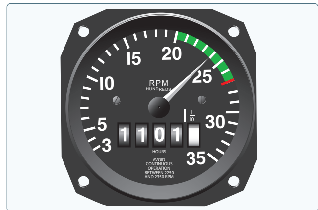
Figure 9-4. Manifold pressure gauge (top) and tachometer (bottom).
