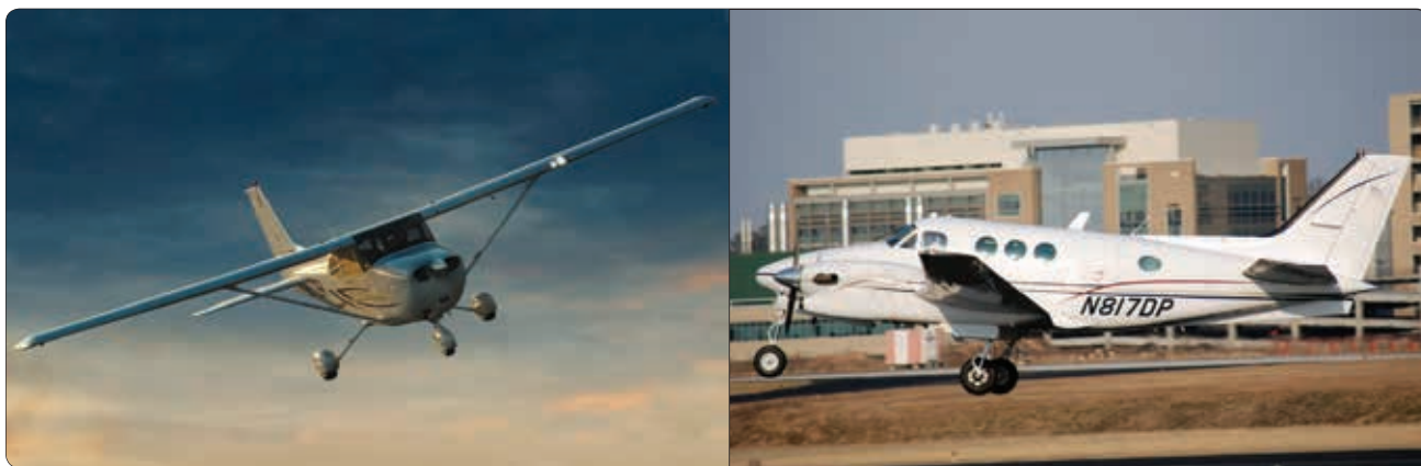
Figure 7-39. Fixed (left) and retractable (right) gear airplanes.
