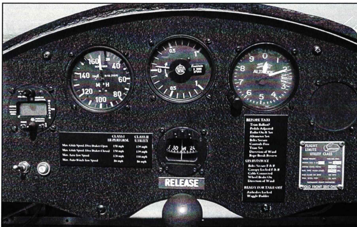
Figure 1.6 – Typical glider instrument panel, with (from L to R) a radio, an airspeed indicator, a variometer, an altimeter, and a compass (lower center).
