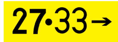
Figure I. Destination Sign for common taxiing route to two runways
