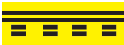
Figure M. Runway Boundary Sign
