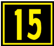
Figure G. Runway Location Sign
