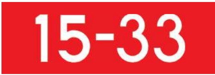
Figure A. Runway Holding Position Sign
