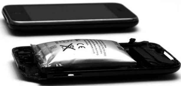
Figure 10-1. Damaged LiPo battery with bulging exterior coating (Mpt-matthew; https://en.wikipedia.org/wiki/File:Expanded_lithium-ion_polymer_battery_from_an_Apple_iPhone_3GS.jpg ; CC BY-SA 3.0)
