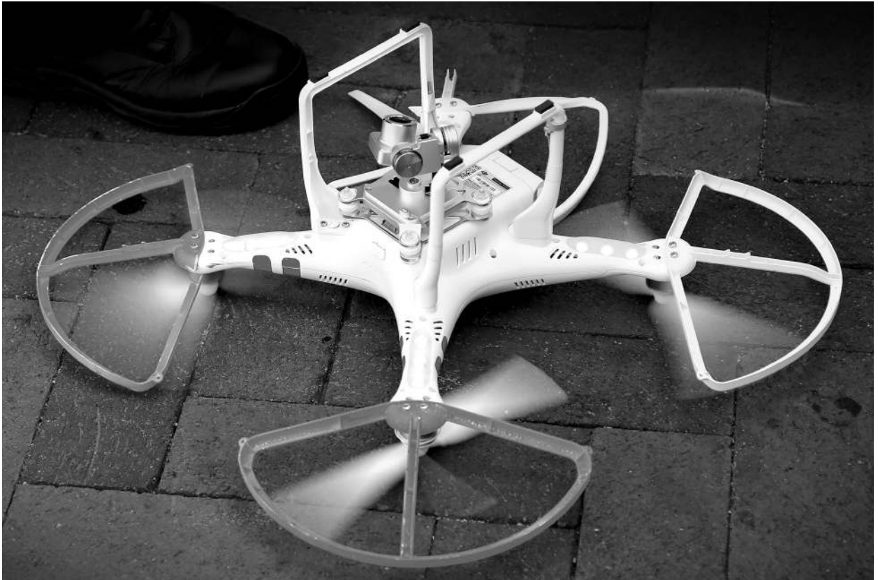
Figure 8-1. This UAS crashed into the ground upside down following a fly-away.
