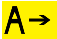
Figure H. Direction Sign for runway exit
