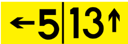
Figure J. Destination Sign for different taxiing routes to two runways
