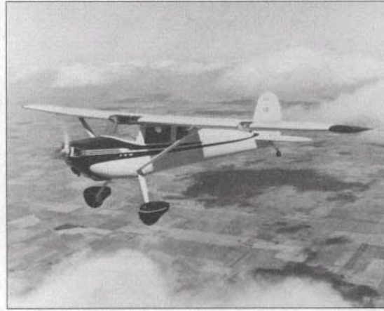
The Cessna 140 was a deluxe two-seat airplane with a cruise speed of over 100 m.p.h. The first 140s were delivered in 1946, but the spunky little plane is still in huge demand by pilots who often go to compulsive efforts to restore them to their original charm.
