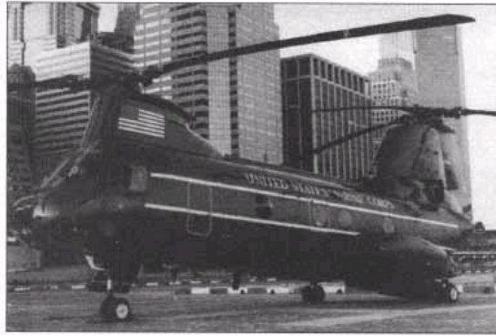
Helicopters like this CH46E Sea Knight use two main rotors rather than one, eliminating the need for an antitorque rotor and increasing the amount of weight it can carry. (U.S. Marine Corps photo)
