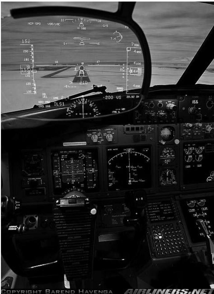
Figure 8.2 Head-up display during a landing
