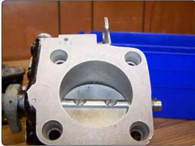
Figure 2-14. Throttle action in idle position.
