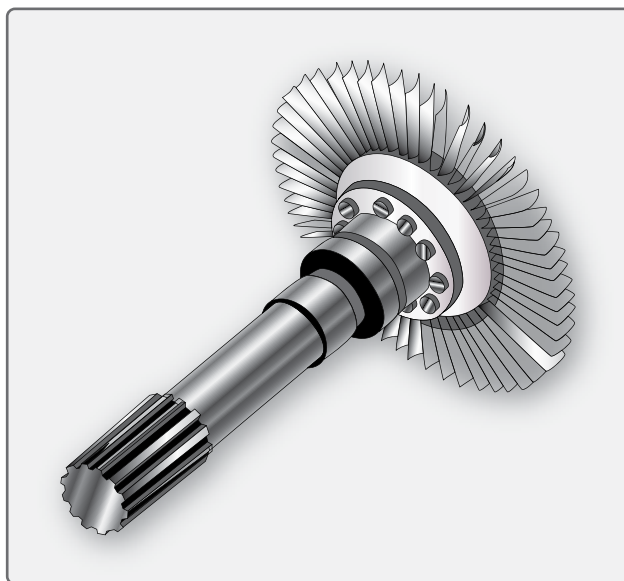
Figure 1-63. Rotor elements of the turbine assembly.
