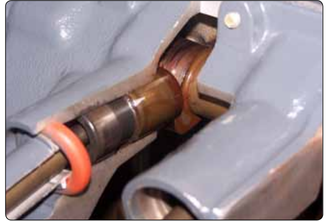
Figure 1-29. Cam load on lifter body.
