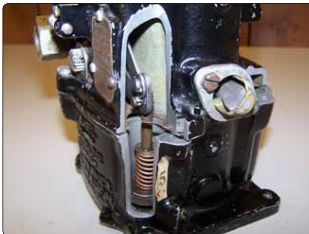
Figure 2-19. Accelerating pump shown in cutaway.
