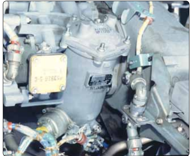
Figure 2-60. Dual element fuel pump.
