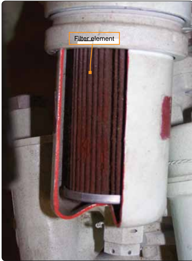
Figure 6-35. Turbine oil filter paper element.
