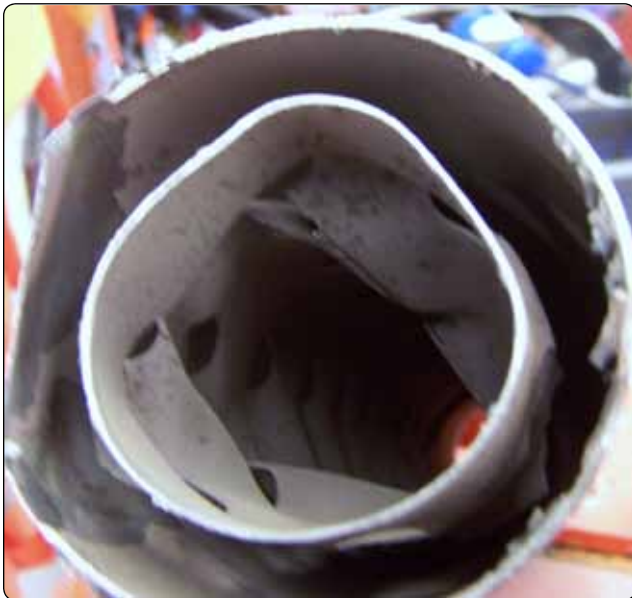
Figure 3-43. An example of internal muffler failure. Muffler failure can be caused by erosion and carbonization, which in turn can lead to breakage blocking exhaust flow.
