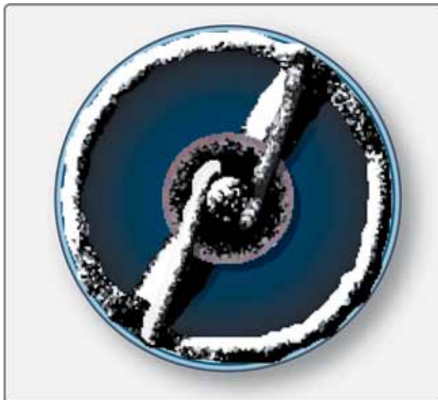
Figure 4-48. Carbon fouled spark plug.
