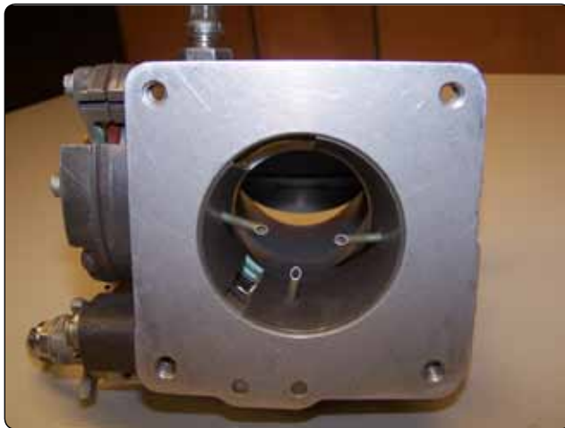
Figure 2-32. Impact tubes for inlet air pressure.
