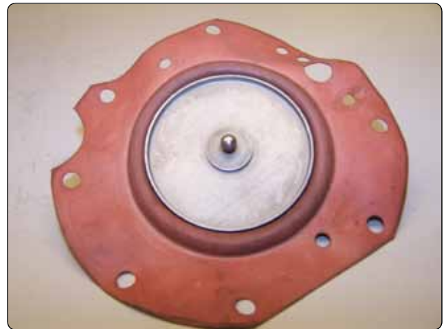
Figure 2-33. Fuel diaphragm with ball valve attached.
