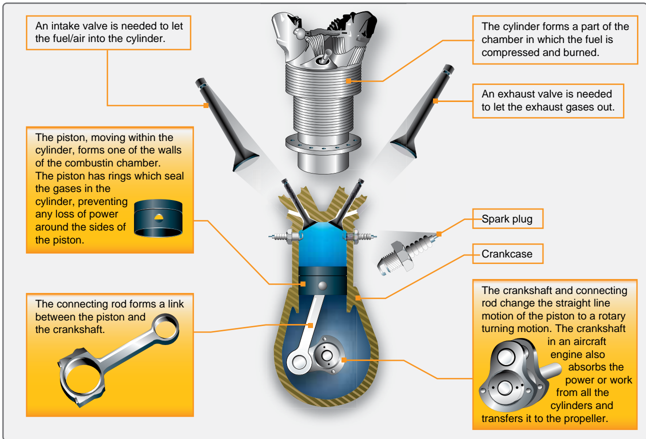
Figure 1-4. Basic parts of a reciprocating engine.
