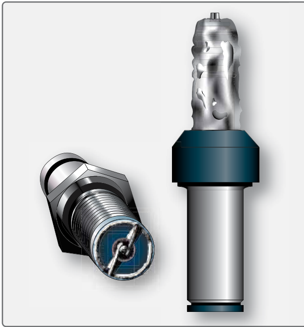
Figure 4-49. Lead fouled spark plug.
