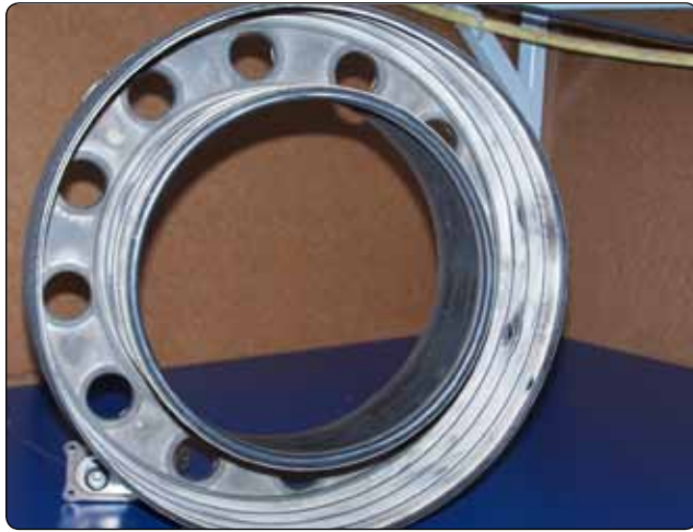
Figure 1-58. Annular combustion with chamber ceramic coating.
