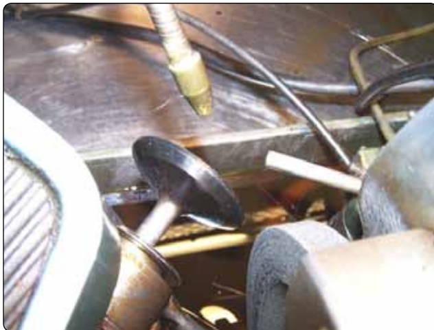
Figure 10-25. Valve in chuck ready to grind.
