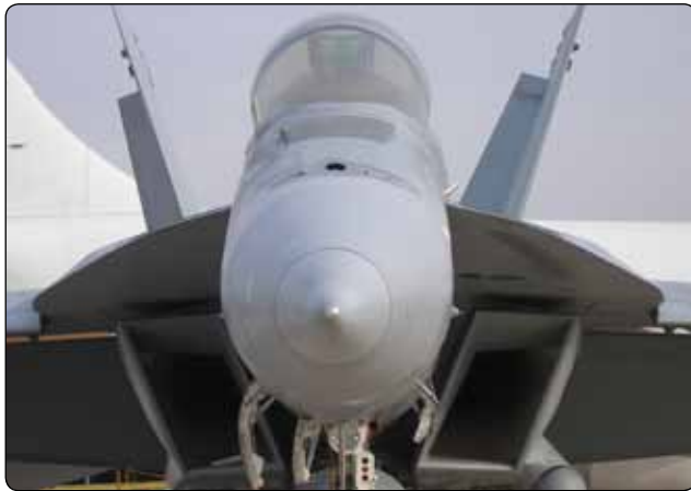
Figure 3-25. An example of a divided-entrance duct.
