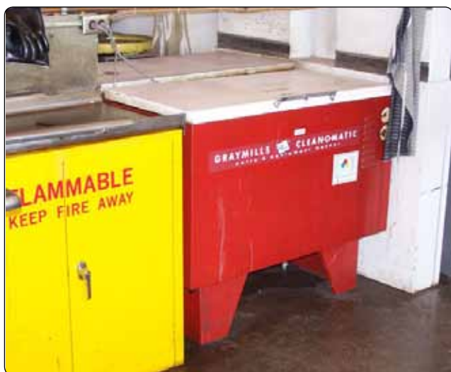
Figure 10-3. Typical solvent degreasing tank.
