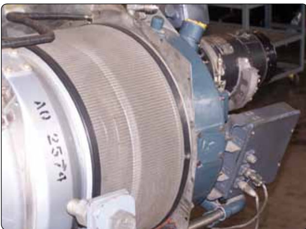
Figure 3-28. An example of a turboprop engine that incorporates inlet screens.
