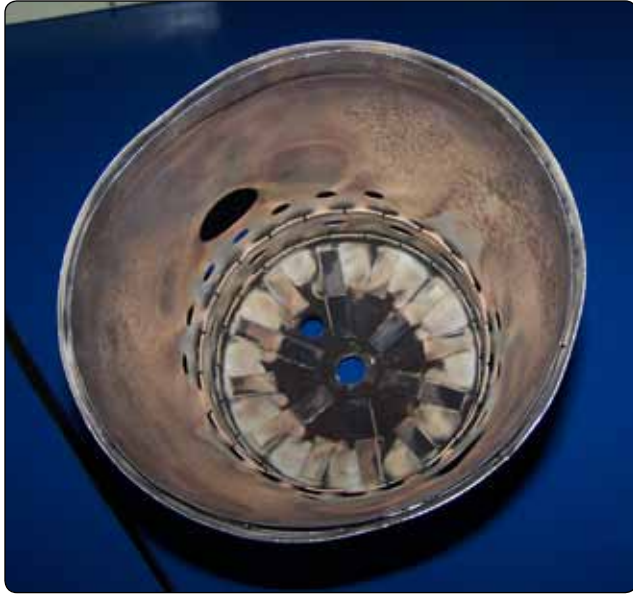
Figure 1-53. Inside view of a combustion chamber liner.
