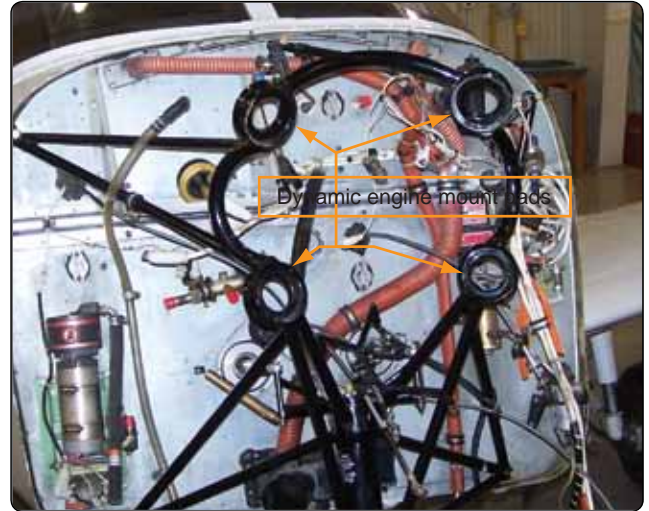
Figure 8-16. Rubber shock mount in steel engine mount.
