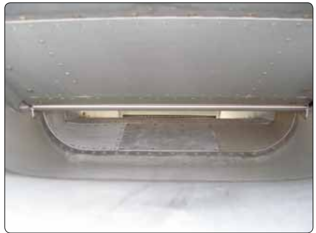
Figure 3-33. Deflector doors used to deflect ice or dirt away from the intake.
