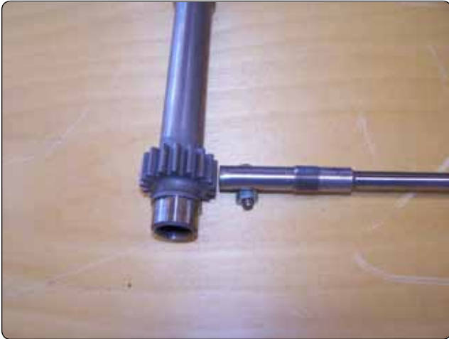
Figure 10-79. Magnetic pickup and gear.
