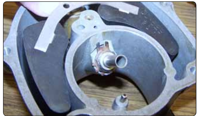
Figure 2-9. Float chamber discharge nozzle and float.
