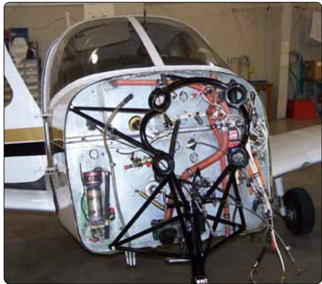
Figure 8-2. Typical firewall with components mounted on it.
