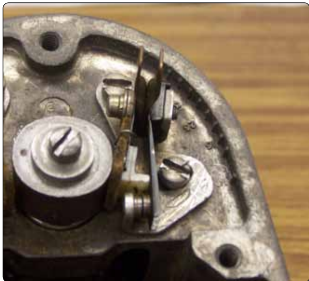
Figure 4-8. Pivotless type breaker assembly and cam.
