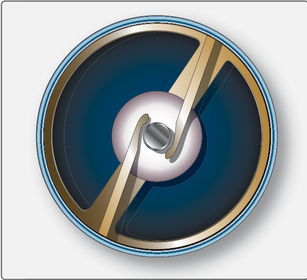
Figure 4-50. Spark plug gap erosion.
