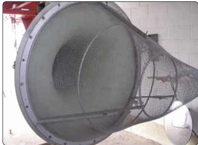
Figure 3-30. A bellmouth inlet used during system tests.
