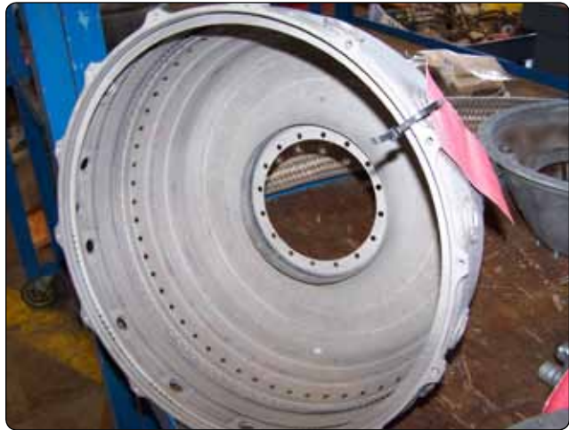
Figure 10-63. Combustion case inspection.
