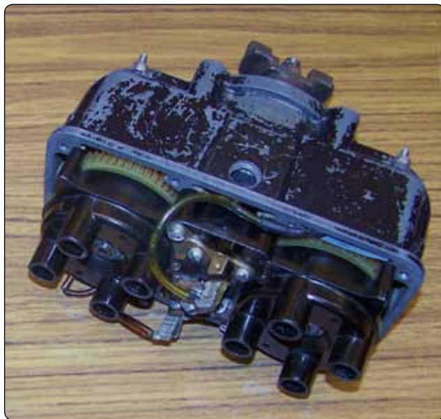
Figure 4-18. A dual magneto with two distributors.
