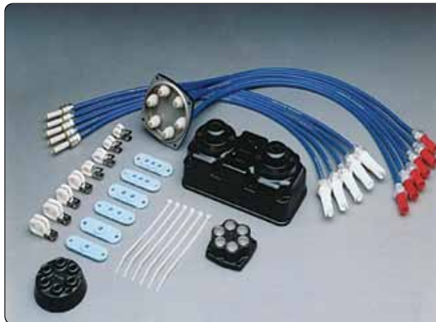
Figure 4-11. A high-tension ignition harness.
