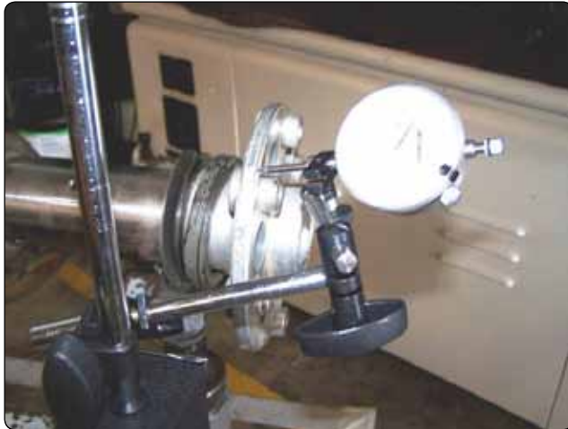
Figure 10-10. Checking crankshaft runout.
