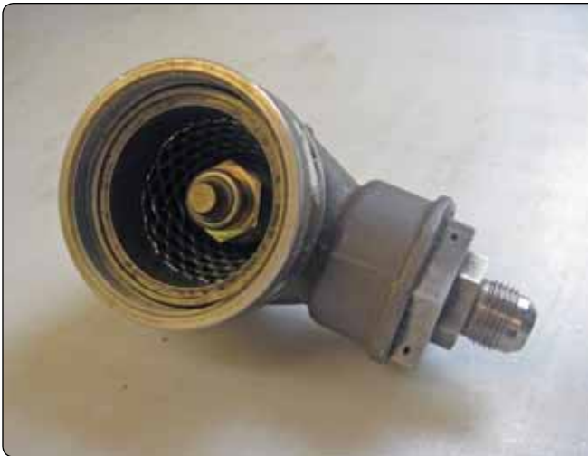
Figure 9-10. Discharge valve and cartridge (squib).
