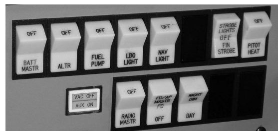
Figure 9.2 (a) Switch configurations, (b) rocker switches
