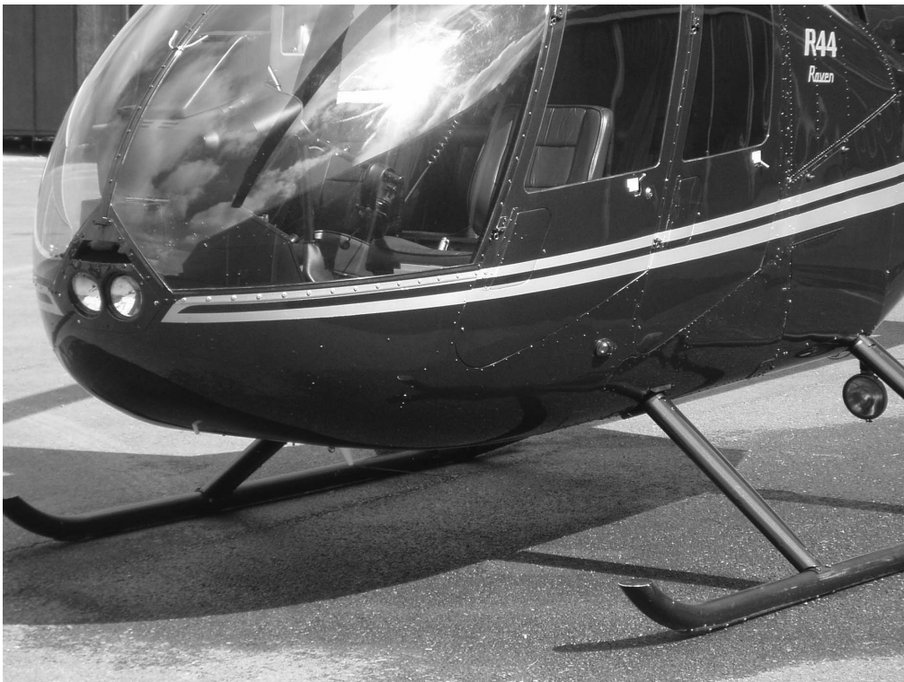
Figure 12.21 Helicopter lights: Twin landing lights on nose; Navigation light below door; Additional landing light on rear skid
