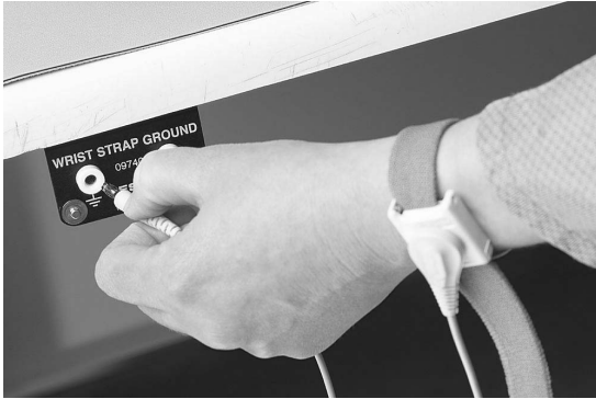
Figure 20.22 ESD Typical wrist strap grounding point
