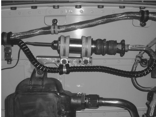
Figure 16.9 Responder located in the engine fire zone
