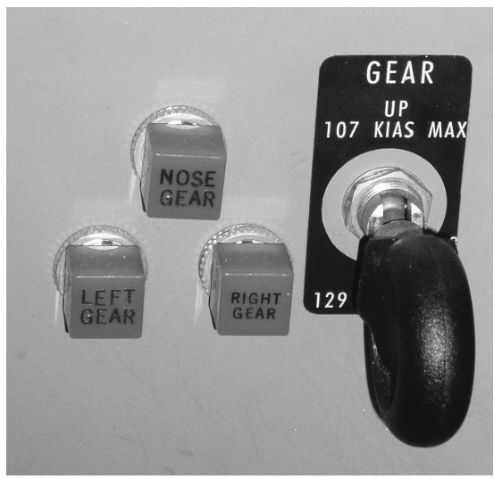
Figure 14.2 Landing gear position indication: (a) system schematic, (b) typical gear position selector and warning lights (general aviation)
