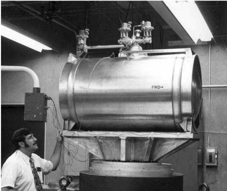
Figure 10.1 The C-5A LN 2 dewar during vibration testing (courtesy of Parker Aerospace).
