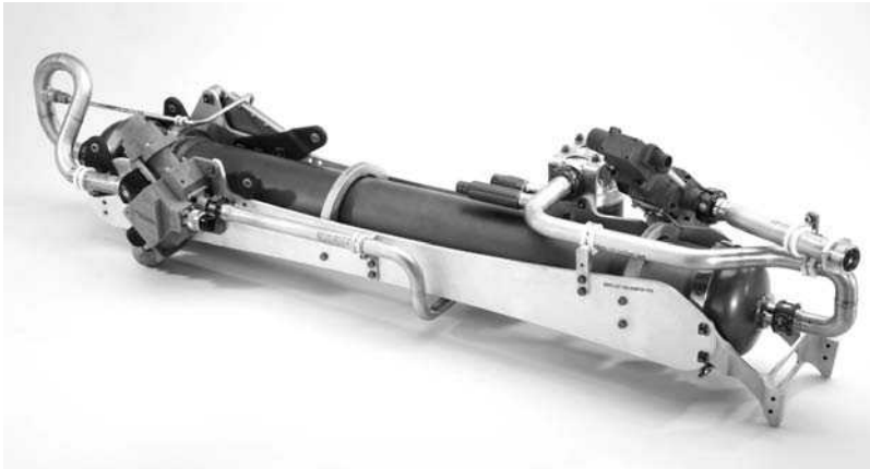
Figure 10.9 Airbus A320 Inerting system demonstrator (courtesy of Parker Aerospace).
