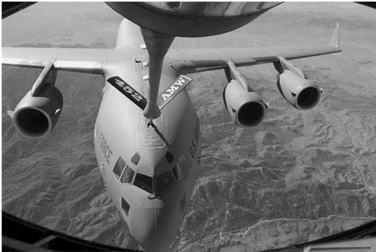
Figure 5.9 A C-17 being refueled via the flying boom (courtesy of US Air Force/Master Sgt. Rick Starza).
