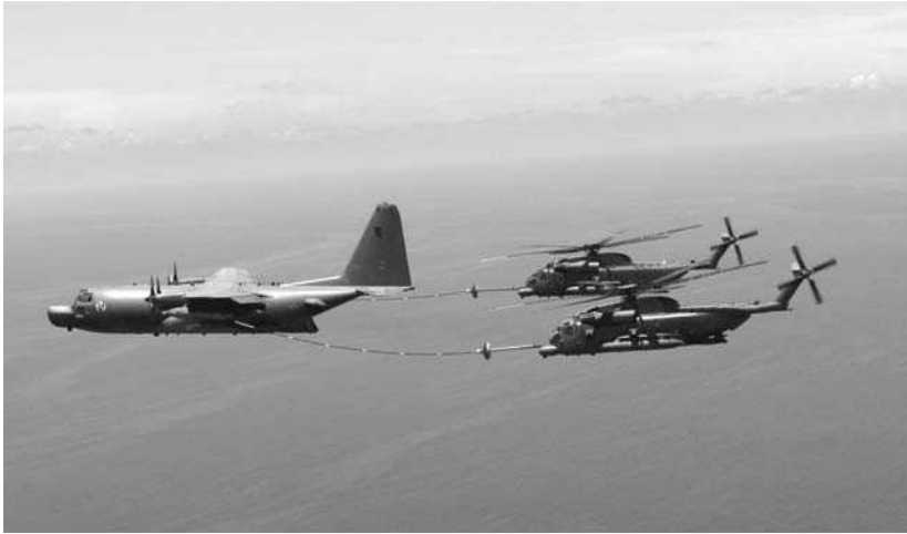
Figure 5.15 Aerial Refueling of MH-53 Helicopters (courtesy of US Air Force/Senior Airman Emily Moore).
