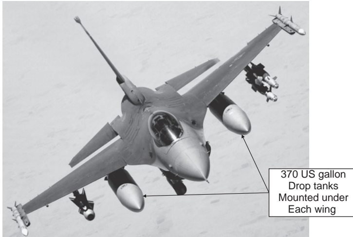
Figure 3.20 F-16 with drop tanks (courtesy of US Air Force/Master Sgt. Andy Dunaway).
