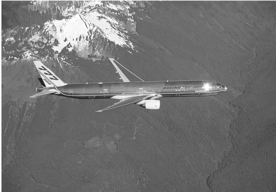
FIGURE 1 The Boeing 777. A long-range (8200 mi), wide-body, Mach 0.85 transport with 300 passengers, two high-bypass-ratio turbofans of the 90,000-lb thrust class, a maximum gross weight of 630,000 lb, a wing area of 4600 ft 2 ( W/S = 137 lb/ft 2 ), and an aspect ratio ( AR ) of 8.7. [Courtesy of Boeing.]
