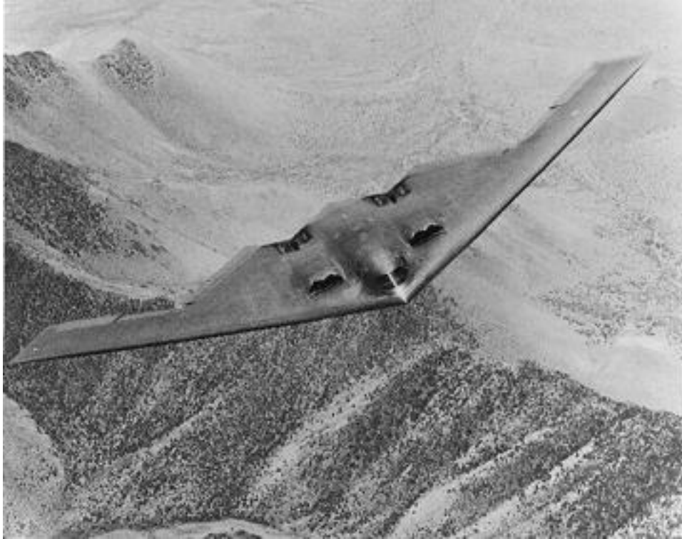
FIGURE 11 The B-2 Spirit (the STEALTH Bomber), originally manufactured by the Northrop Corporation. A high-subsonic-flying wing with multirole missions, a crew of two, four high-bypass-ratio turbofans of the 18,000-lb class, and a typical maximum weight of 335,000 lb. [Courtesy of the U.S. Air Force.]
