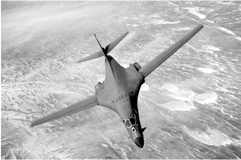
FIGURE 10 The B-1B Lancer, originally built by Rockwell International. A low-level penetration strategic bomber with a Mach 1.2 capability, a crew of four, a swing wing, four low-bypass turbofans of the 31,000-lb (unaugmented) thrust class, and a maximum gross weight of 470,000 lb. [Courtesy of Boeing.]
