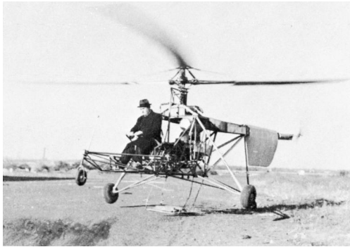
FIGURE 4 Igor Sikorsky at the controls of his single rotor–tail rotor helicopter, the VS-300, December 1941. [Courtesy of The Smithsonian Institution.]
