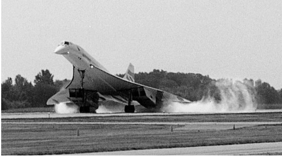
FIGURE 2 The Concorde SST, the only civil supersonic transport (in service for over 30 years). A medium-range, Mach 2.0 transport with 100 passengers, four afterburning turbojets of 38,000-lb unaugmented thrust, a maximum gross weight of 408,000 lb, a wing area of 4134 ft 2 ( W/S = 98.6 lb/ft 2 ), and an AR of 1.7. [Courtesy of British Aerospace.]
