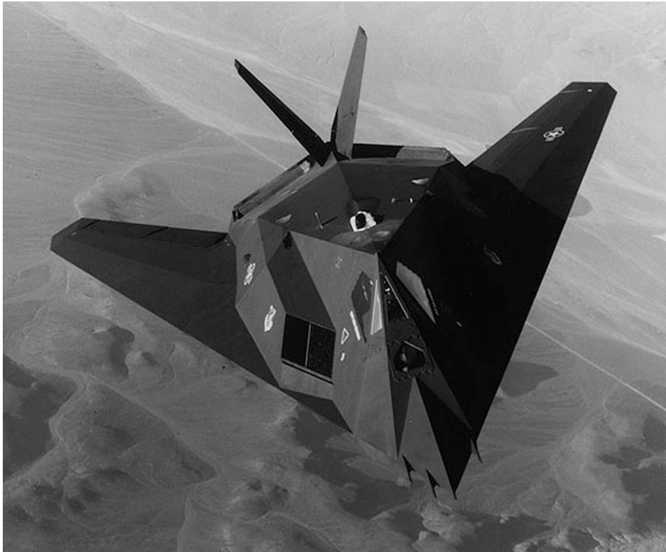
FIGURE 12 The F-117A Nighthawk, a high-subsonic, defense suppression aircraft with a crew of one, low detectability, internal weapons storage, two turbofan engines of the 12,000-lb thrust class, and a weight of 52,000 lb. [Courtesy of Lockheed Martin.]
