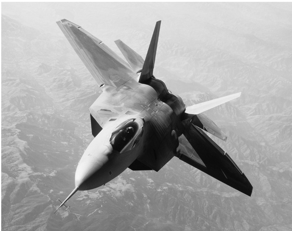
FIGURE 3 The F-22 Raptor, a joint Lockheed Martin/Boeing aircraft. A single-place, Mach 2, air-dominance fighter with two low-bypass turbofans of the 35,000-lb class with supercruise capability, a wing area of 840 ft 2 , and an AR of approximately 2.3. [Courtesy of Boeing.]
