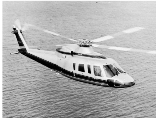
FIGURE 6 Modern, turbine-powered executive helicopter, the Sikorsky S-76.
