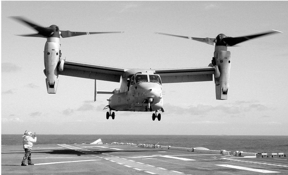
FIGURE 9 The Bell Boeing V-22 Osprey landing on the deck of an assault carrier. A military tiltrotor V_{STOL} (vertical and short takeoff and landing) transport with a capacity of 24 combat troops, two 6150-SHP turboshaft engines, a maximum vertical takeoff weight of 47,000 lb, and a maximum airspeed of 315 mph. [Courtesy of Bell Boeing.]
