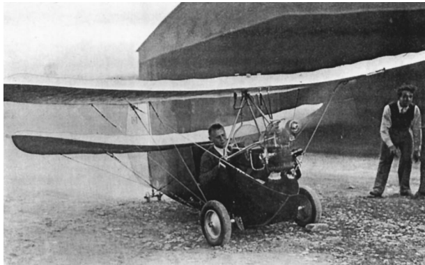
FIGURE 7 The French Le Pou du Ciel ( Flying Flea ), designed by Henri Mignet in the early 1930s, took the aeronautical world by storm and remains the progenitor of all popular home-built projects. Three design faults led to the original being banned. Once the faults were rectified, later modified variants continued to fly and are still among the safest handling and least complicated of all light airplanes. [Courtesy of former Sampson Low, Marston & Co., Ltd., circa 1934–5.]
