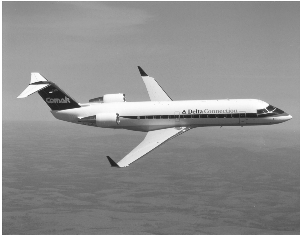
FIGURE 8 The Canadair Regional Jet, CRJ 200. A 50-passenger, Mach 0.81 transport with two turbofans of 8700-lb thrust, a gross weight of 53,000 lb, a wing area of 520 ft 2 ( W/S = 102 \text{ lb/ft}^2 ), and a range of 2300 miles. [Courtesy of Bombardier Aerospace.]
