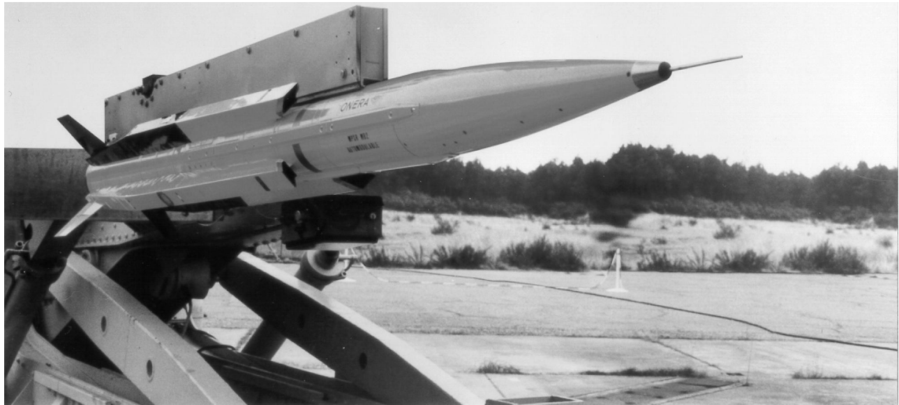
FIGURE 23 View of an MPSR demo missile with a rustique ducted rocket.
