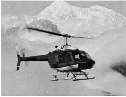
FIGURE 8 Modern, turbine-powered utility helicopter, the Bell 206B Jet Ranger.
