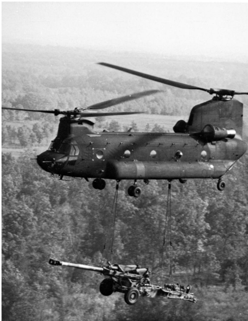
FIGURE 9 Large, tandem-rotor helicopter, the Boeing CH-47 Chinook.
