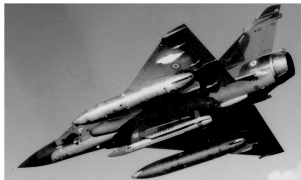
FIGURE 5 Aerospatiale ramjet-powered ASMP nuclear missile carried by Mirage 2000, operational in French forces since 1986 (CEV photo).
