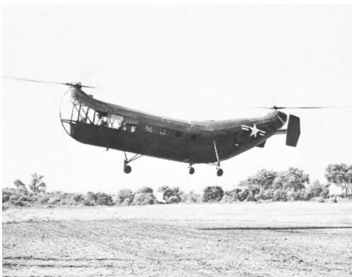
FIGURE 5 First successful tandem-rotor helicopter, the XHRP-X, with its designer Frank Piasecki at the controls.
