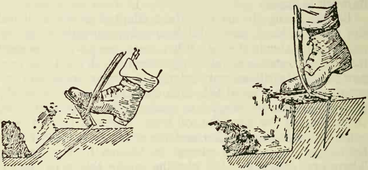
Fig. 46. Wrong and right ways to dig.
