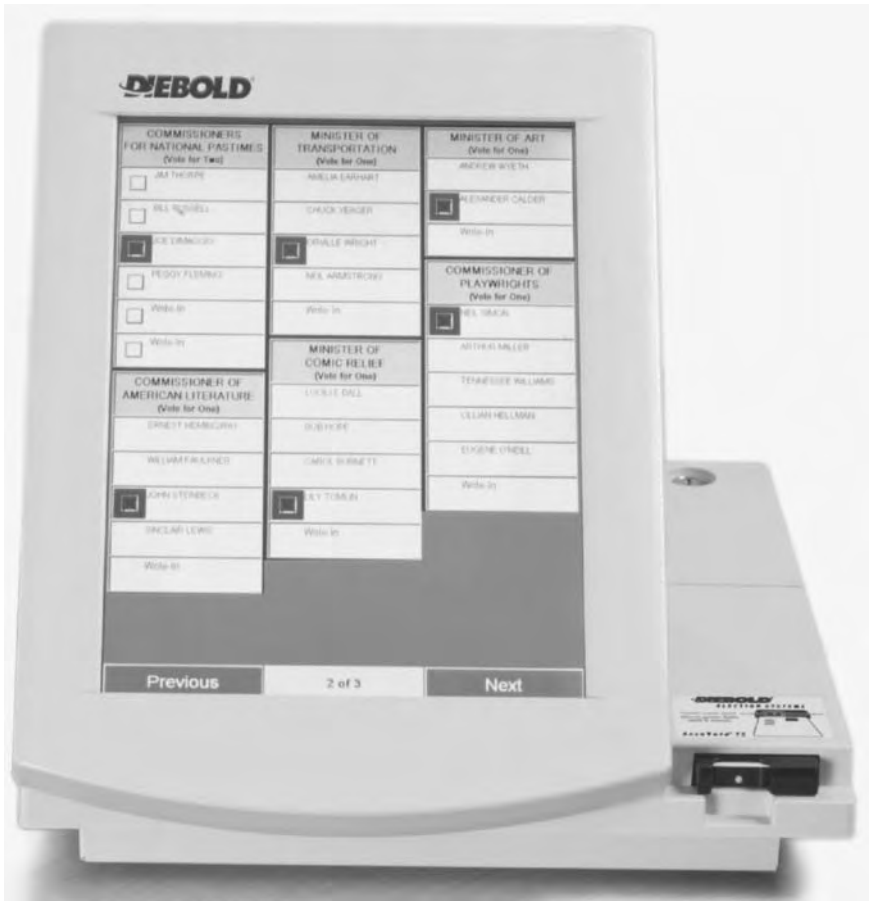
Figure 7.1 AccuVote-TS direct recording touchscreen voting machine, in use ca. 2002. Manufactured by Diebold, Incorporated, North Canton, OH. The touchscreen shows three columns of contests. Each contest is headed by a dark rectangle stating the name of the office. Candidates are listed in series in the whiter rectangles under the office title. The smaller darker squares indicate selections by a voter. The original photograph shows colors. The slot to the lower right of the screen is for entry of the voter's smartcard.
