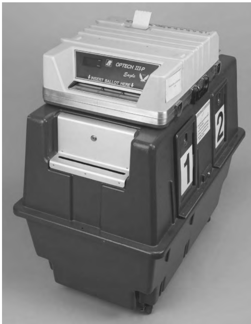
Figure 6.1 Optech III-P Eagle optical scan voting machine and ballot box, in use ca. 2000. Manufactured by Sequoia Voting Systems, Oakland, CA.
