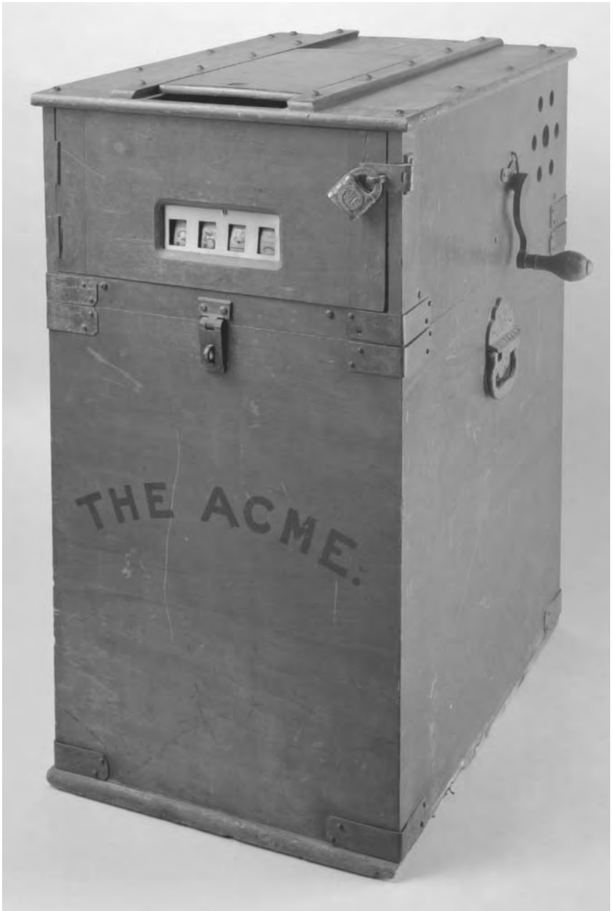
Figure 4.2 Counting ballot box, ca. 1880s. This box has a lever mechanism that accepts one ballot per voter into the box and counts the ballot at the same time. It was manufactured in East Bridgewater, CT.
