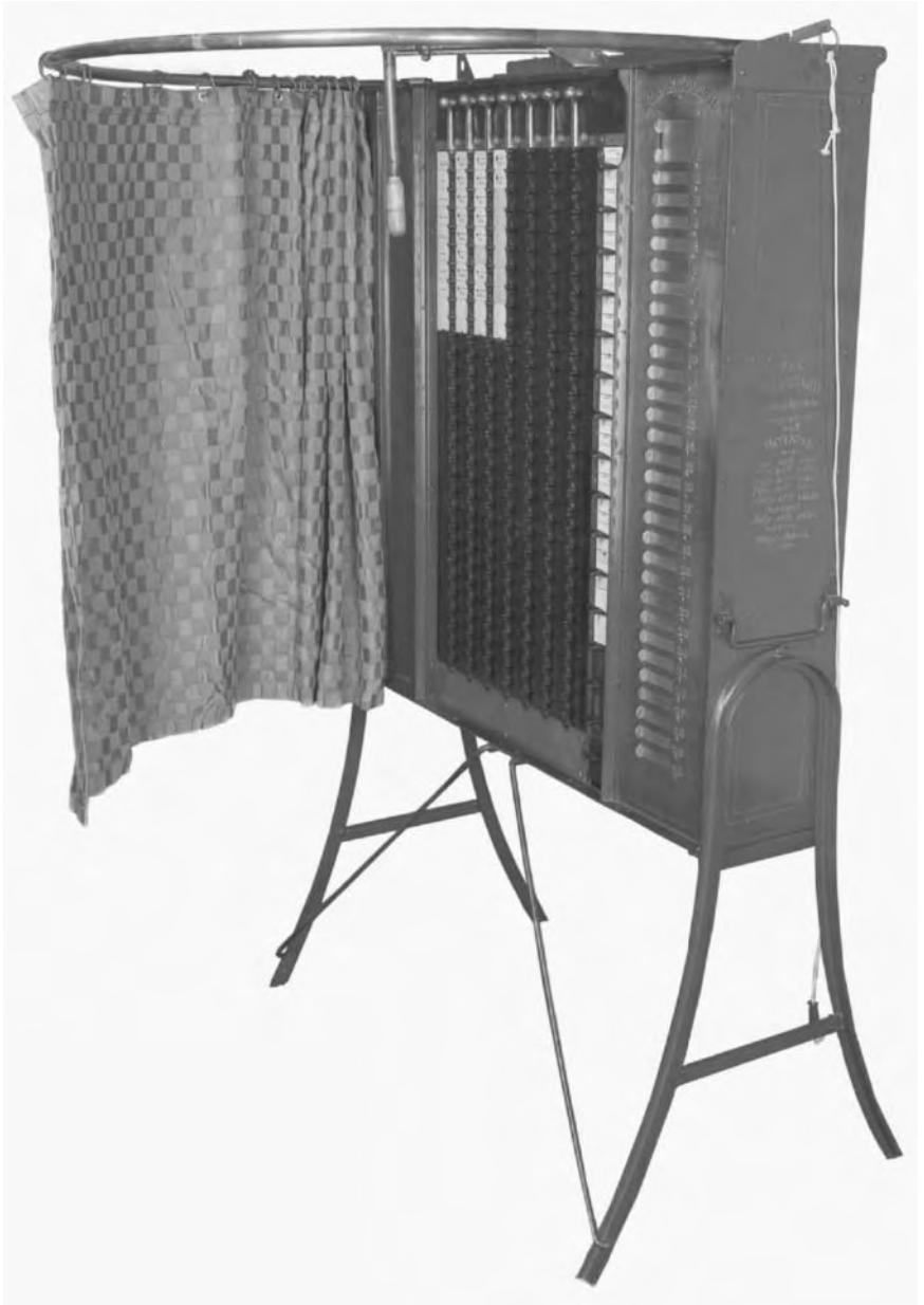
Figure 4.3 Lever voting machine, ca. 1899. Manufactured by the Standard Voting Machine Company of Rochester, NY. Alfred Gillespie invented the procedure in which the large “vote” lever first closes the curtain for privacy and opens it while registering the votes at completion of voting.
