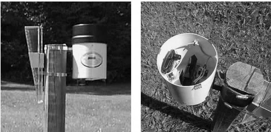
Figure 6.1 Recording rainfall logger is mounted beside a total rainfall gage. The picture on the right shows the tipping bucket and event recorder ( www.onsetcomputer.com ) (T. Seybert).
