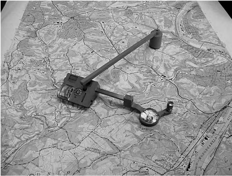
Figure 5.5 Polar planimeter used for measuring area (T. Seybert).
