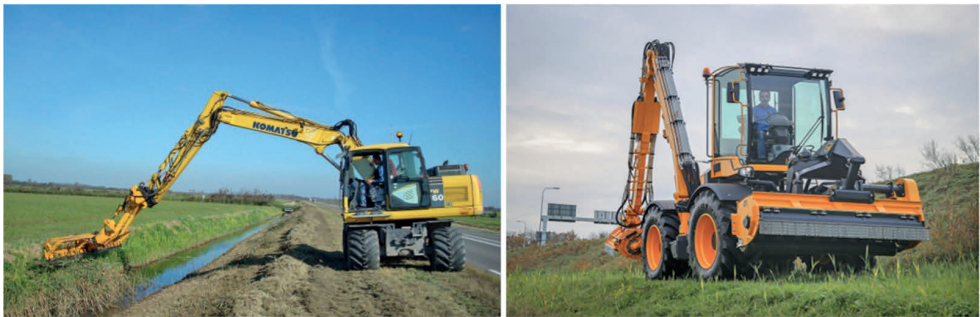
Figure 24.3 Weed clearance machinery. Drain cleaning by tractor mounted mowing bucket and the self-contained Herder One (on the right) with rotating cabin, mowing bucket and flail mower, or crash barrier mower or the weed brusher. (from Herder BV Brochure 2019, www.herder.nl/en/herder-one/ )
