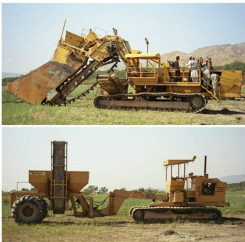
Figure 8.17 Trencher and gravel hopper (photographs W.F. Vlotman)
