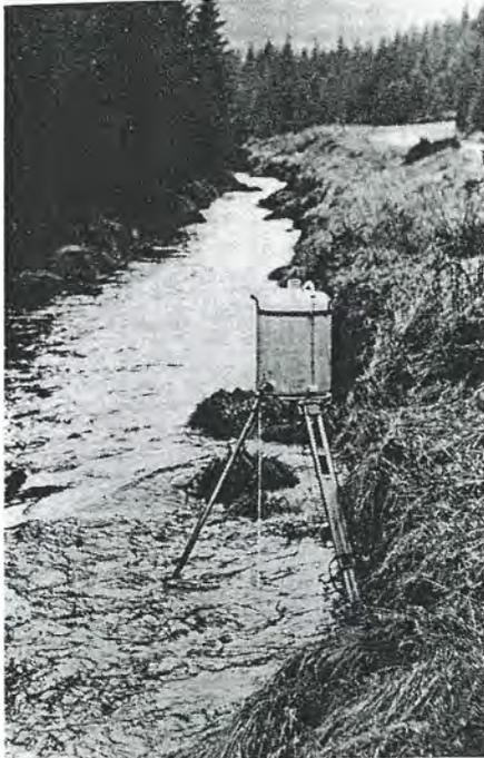
Fig. 2.9a. Discharge measuring by chemical dilution method (by courtesy of CIRIA, London).
