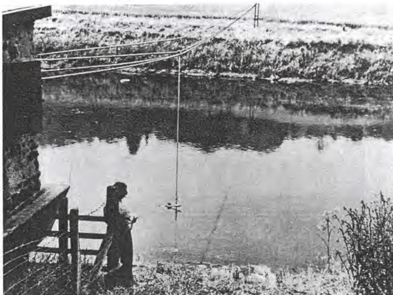
Fig. 2.12b. Permanent cable station (by courtesy of CIRIA, London).
