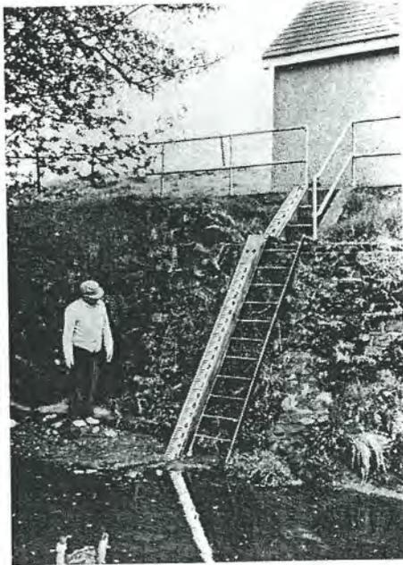
Fig. 2.1c. Inclined staff gauge (by courtesy of CIRIA, London).
