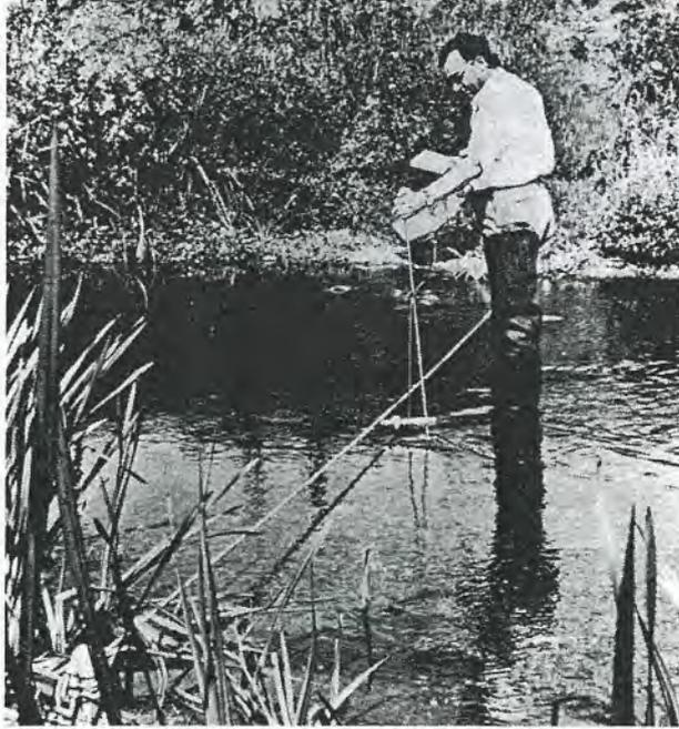
Fig. 2.11 a. Measurement by wading (by courtesy of CIRIA, London).
