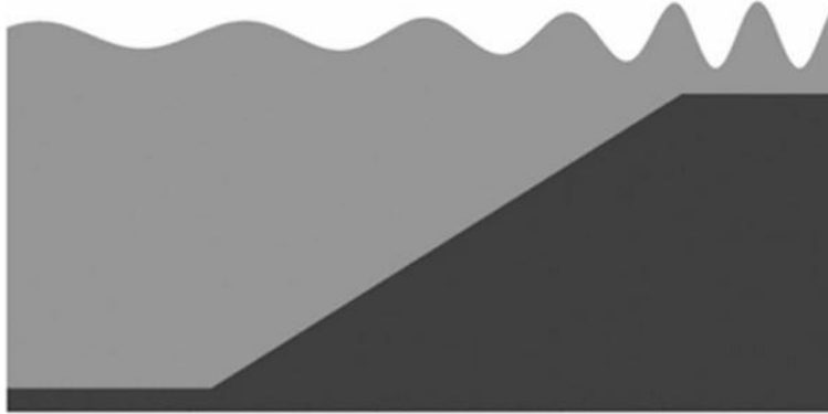
Figure 14.4 Tsunami wave transformation as it enters shallow water. (Source: http://en.wikipedia.org/wiki/Tsunami_Generation_mechanisms )
