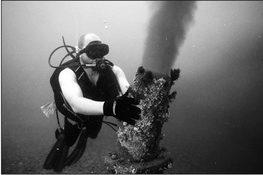
Figure 4-8 Perth desalination plant discharge diffuser – rhodamine dye test
