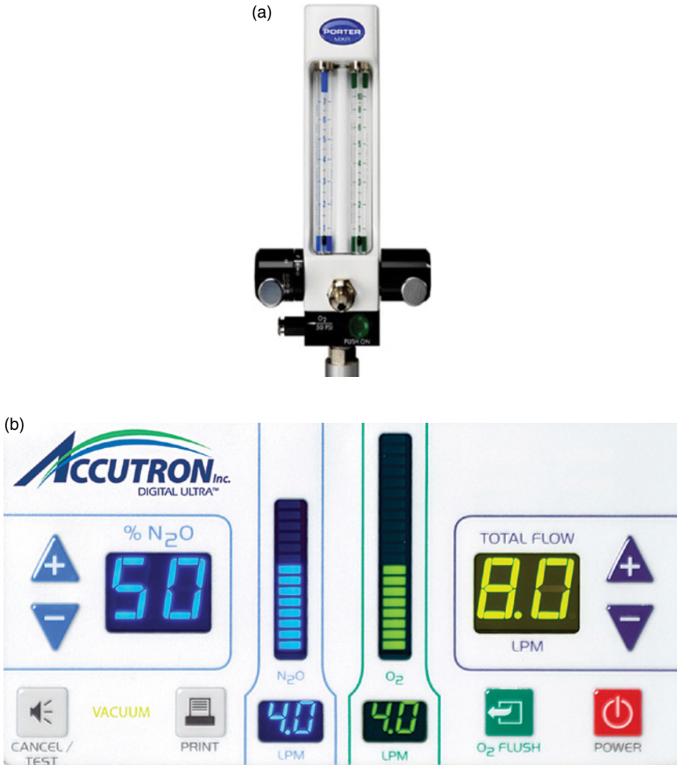
Figure 7.6 (a) Nitrous oxide ball float. (b) Digital flow meter.
