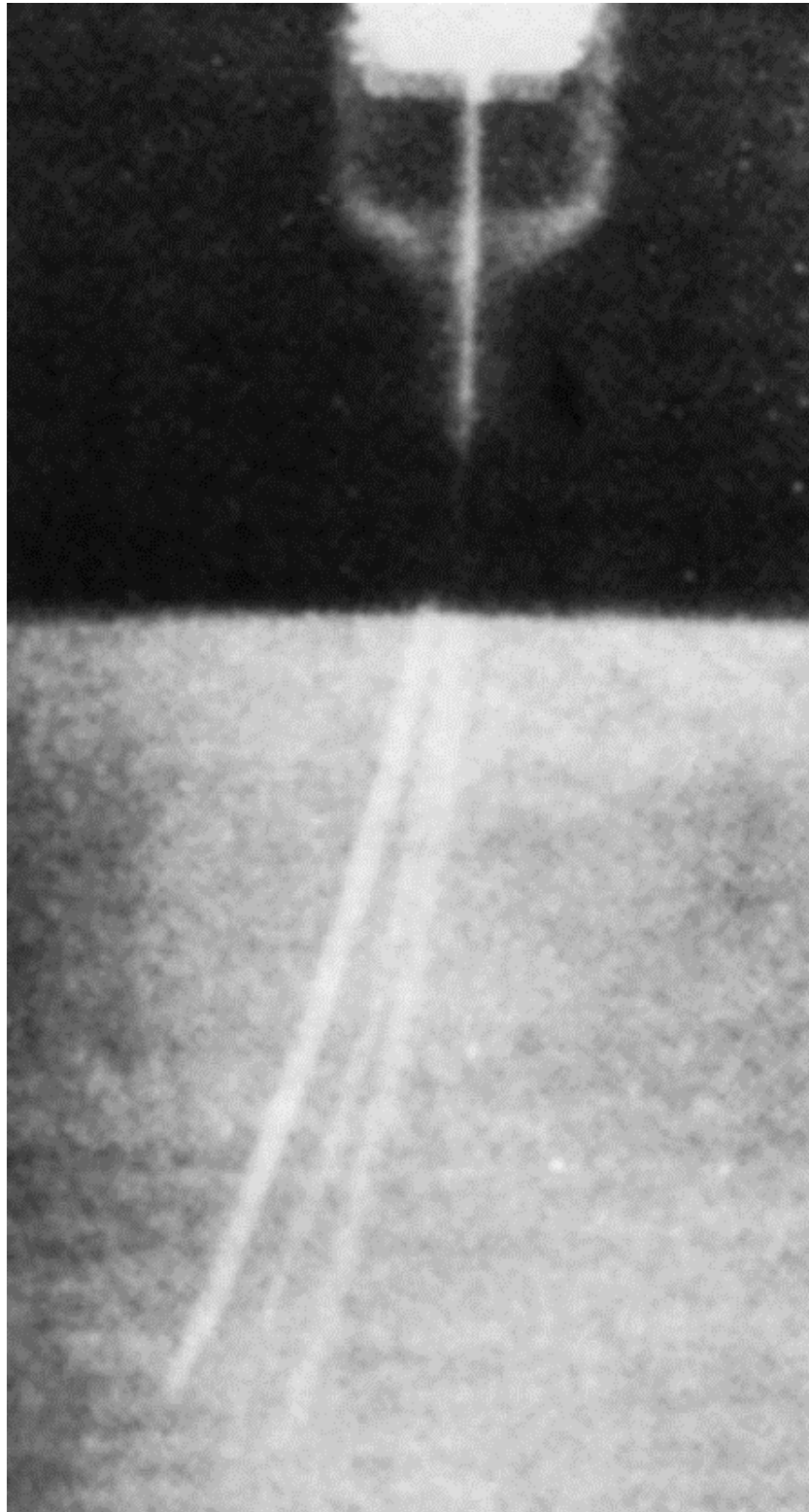
Figure 6-3 Radiograph demonstrating varying degrees of needle deflection with different gauges ( left to right, 30-, 27-, and 25- ).
