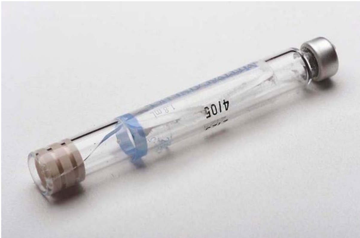
Figure 7-11 Cracked glass on dental cartridge.
