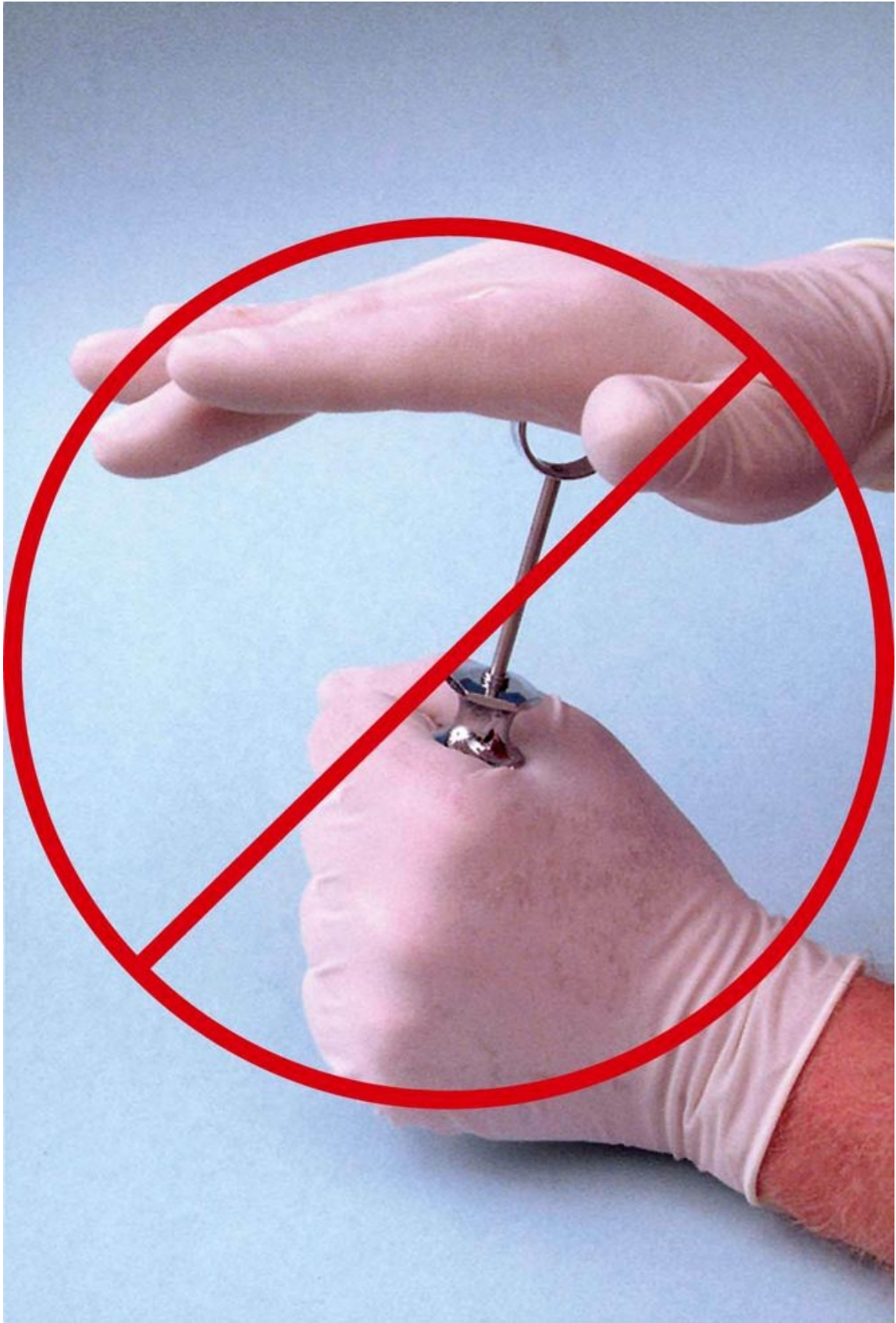
Figure 9-5 Do not exert force on the plunger; the glass may crack.
