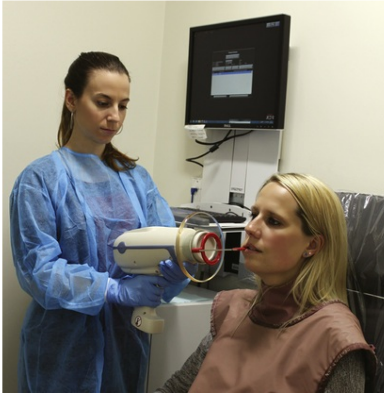
FIG. 7.31 Handheld x-ray machine for intraoral radiography. Operator dose is minimized by a shield on the aiming cylinder to reduce backscatter. (Courtesy Dr. Akrivoula Soundia and Dr. Holly Vreeburg, UCLA School of Dentistry, Los Angeles, CA.)
