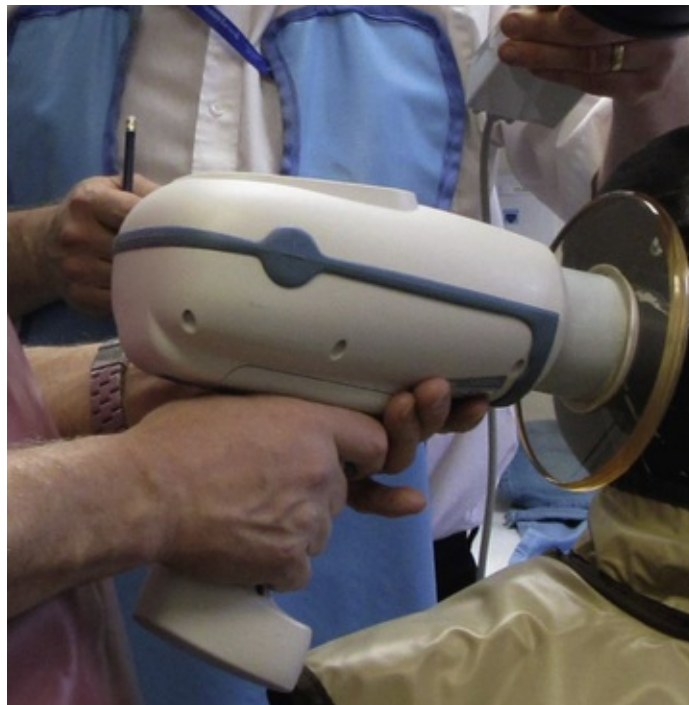
FIG. 33.8 Example of a handheld dental x-ray generator.
