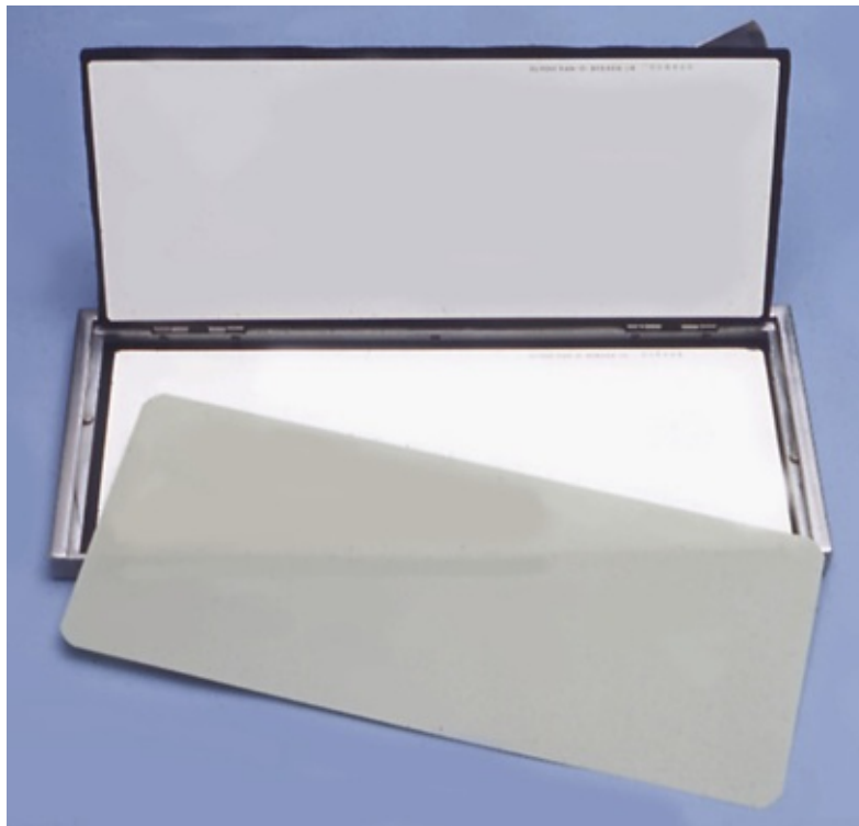
FIG. 5.8 Cassette for 8-Inch × 10-Inch Film Along With a Sheet of Screen Film. When the cassette is closed, the film is supported in close contact between the two white intensifying screens seen on the inside of the cassette. These intensifying screens absorb most of the incident x-ray beam and then fluoresce and expose the film.
