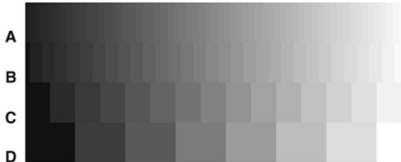
FIG. 4.9 Contrast Resolution. Examples of gray-scale ramps representing distinct gray levels from black to white. Bit depth controls the number of possible gray levels in the image. The actual number of distinct gray levels that are displayed depends on the output device and image processing. The perceived number of gray levels is influenced by viewing conditions and the visual acuity of the observer. (A) 6 bits/pixel = 64 gray levels. (B) 5 bits/pixel = 32 gray levels. (C) 4 bits/pixel = 16 gray levels. (D) 3 bits/pixel = 8 gray levels.
