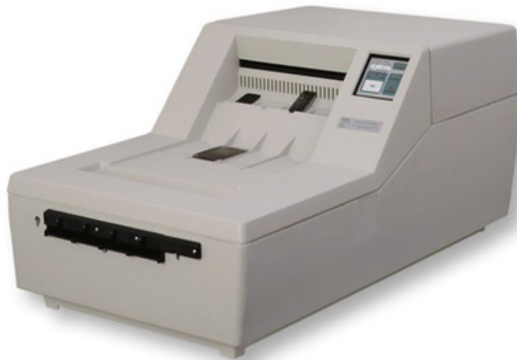
FIG. 5.20 Dent-X 810 AR Film Automatic Film Processor. The operator opens the film packet in a darkroom and inserts the film into the opening on the left end of the machine. The exposed film is carried on a roller apparatus through processing solutions, and the processed and dried film is returned through the upper right opening in 4.5 minutes. (Courtesy ImageWorks, Elmsford, NY.)
