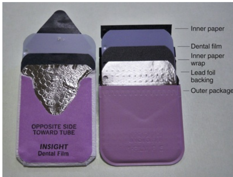
FIG. 5.4 Moisture-proof and lightproof packets, paper on the left and vinyl on right, contain an opening tab on the side opposite the tube. Inside is an interleaf paper wrapper that is folded around the film as well as a sheet of lead foil. Film is packaged with one or two sheets of film. The foil is positioned between the back side of the packet and the paper wrapper. In this position, it absorbs radiation that has passed through the film and prevents scatter radiation from blurring the image. If the film packet is inadvertently placed backward in the patient's mouth, the mottled image of the foil shows on the resultant image. (Courtesy of Carestream Dental, a division of Carestream Health, Inc., Atlanta, Georgia.)
