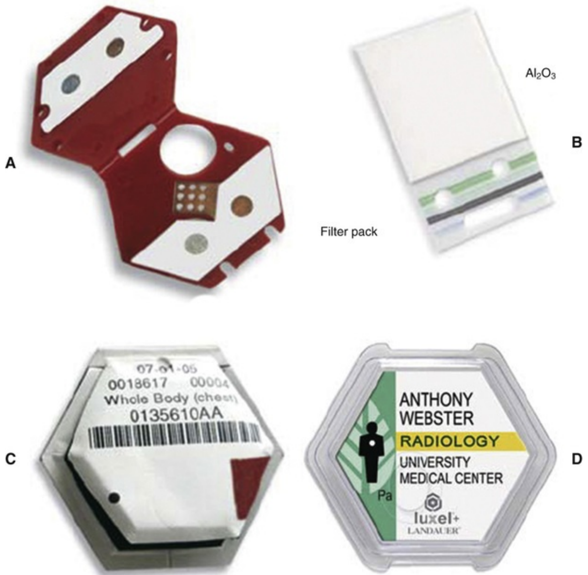
FIG. 3.9 A personal optically stimulated luminescence dosimeter. (A) Filter pack containing an open window and plastic, aluminum, and copper filters. (B) Strip of \text{Al}_2\text{O}_3 , which is sensitive to radiation. (C and D). The filter pack and \text{Al}_2\text{O}_3 , are packaged into blister pack and worn by an operator. The amount and ratio of light output during the stimulation process from the regions of the \text{Al}_2\text{O}_3 under the filters allows determination of the energy and dose of radiation to which the badge was exposed. (Courtesy Landauer, Inc., Glenwood, IL.)
