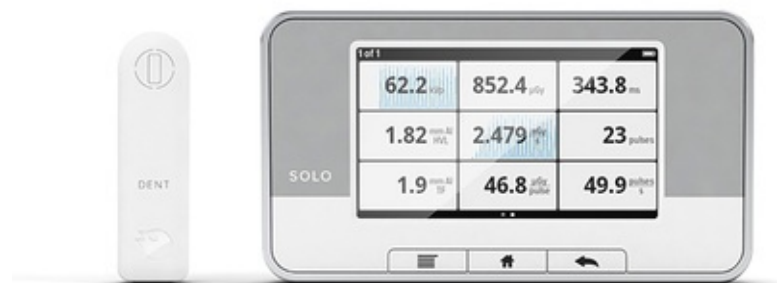
FIG. 16.2 The RaySafe X2 Solo DENT device is designed for dental offices and measures dose, dose rate, kVp, exposure time, pulses, and pulse rate. The sensor can be used for intraoral, panoramic, cephalometric and cone beam computed tomography applications. (Courtesy Fluke Biomedical, www.flukebiomedical.com .)
