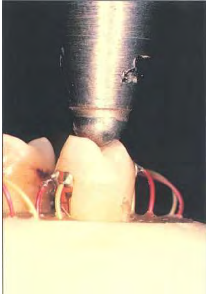
Fig 15-9 Extracted maxillary premolar with strain gauges bonded to the buccal and palatal cusps, subjected to experimental cuspal loading. Nondestructive sequential testing of the effects of cavity preparation and restoration on cuspal flexure is possible with this approach.
