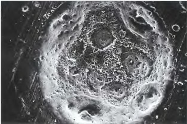
Fig 16-7 Scanning electron micrograph (SEM) of CO 2 laser crater walls appear to be glazed, but the floor is covered with pits (original magnification X100). (Reprinted from Pashley et al. 95 with permission.)
