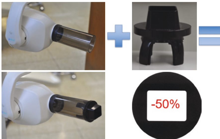
Fig. 1.2 Circular versus rectangular collimation: the retrofitted rectangular collimator enables a radiation dose reduction of approximately 50%
