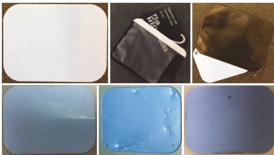
Fig. 1.4 Top row showing clean, undamaged photostimulable phosphor storage plates—bottom row showing damaged and dirty photostimulable phosphor storage plates
