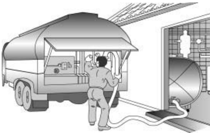
Figure 5.8. Collection of milk on the farm. The tanker is pumping milk from the farm bulk milk tank for transport to the dairy factory. Reproduced with permission from Tetra Pak.
